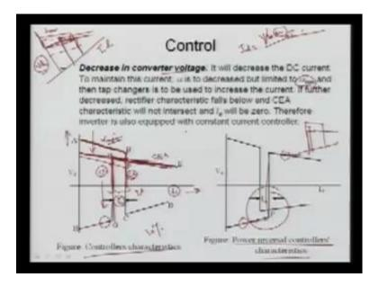
Let us see here what is this, this is your I D, x axis this is the DC voltage your y axis and this is your the constant current control that is your rectifier is doing and this is here your inverter operation here its say CEA. So, here as I was telling that the cc this is your rectifier and this is your inverter is operating other side we will see later why we have made some modification, again let us come to this point.
