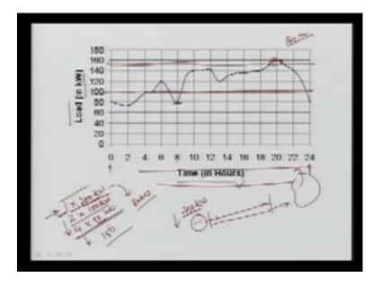
Now, we can see the typical load, just here I have the represented very small amount of load that is in watt at any particular substation. This disturbance substation here, the time in hours starting from 0 that is midnight to here, again we are coming here to the midnight. So, you can see this here the variation keeps on changing and sometimes it is a peak, may even occur in the evening may in mid, it depends upon what type of load you are using.
