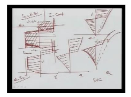
So, the natural characteristic of svc, normally the operating this zone; this is this. And then we have the slope and then this 1. So, here this is operating zone, here we have to operate our SVC is; when voltage is more than reference point then we only we have to go for in this inductive zone, this is your capacitive zone and this capacitive zone, if voltage is less then we have to provide this 1. So, this is your called your current-voltage, that is, VI characteristics of the svc.
