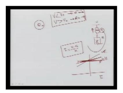
Here again I want to show you that, this reactive power here the supply is 1 objective, means; whenever they are connected, they normally feed reactive power or they can absorb whenever required, means: the stat com or the SVC; they will inject the reactive power at the system, when the voltage is less, when the voltage is less for example, stat com configuration as I showed you here; this is your converter.
