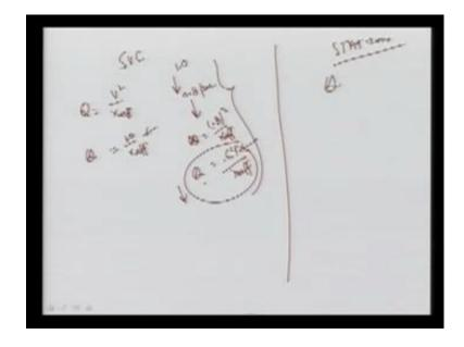
So, the reactive power provided by your SVC it is the v square divided by whatever can say xe or x effective which I am using. Now, you can see if your voltage falls down from 1 per unit to let us suppose 0.8 per unit, when it was 1 per unit it was giving the reactive power at 1 per unit this 1 over x effective. Now, I have this value this x cube will be your 0.8 square divided by x effective and it is 0.6 4 upon x effective what does it mean.
