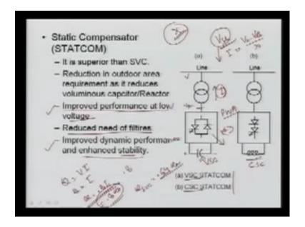
However, another shunt device is your stat com that is called static synchronous compensator or stat com simply. It is superior than SVC the reason that, it is here the converter based technology. If you see in the previous one it was here your thyristor simple anti parallel thyristor it is not a converter. So, it is superior because we are using the converters here, the reduction in the outdoor area requirement it requires less space it
