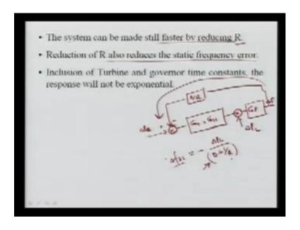
For example, you can see here that is I can say here; this is you're the turbine and governing transfer functions. I can say G T and here we can multiplied by your G H. Then, we are having here your G P if you remember means, this G P is the transfer function of our system including your. And here this is your changing F and that is here coming through 1 over R that is and finally, here that is coming to be here and this is your changing p c and this is here it is negated, this is your positive.
