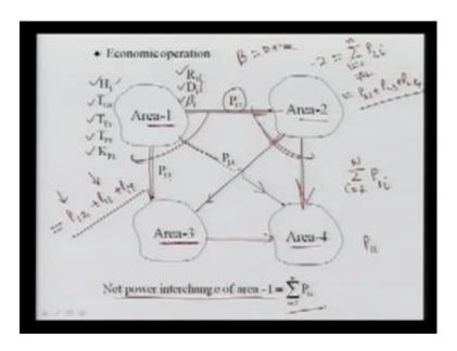
Now, you can see just here shown these 4 area system and all the areas are connected by the tie line. For example, area 1 is connected with area with area 2 with this tie line and the power which is flowing this P12 that is going here. Similarly, this area 1 is connected with area 3 and here power is again the tie line connection and the power is flowing 13. Here we are talking from 1 to 3 it is some value it may be negative or positive.
