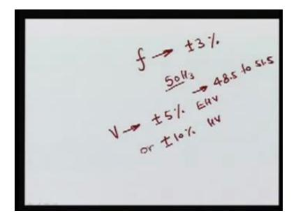
Normally, here the power quality if you achieve in terms of frequency variation, here your frequency of the power system always we operate in the plus minus three percent of the normal rated. So, if we are operating at the 50 hertz here 50 hertz cycle as you
