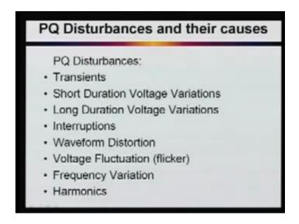
The various PQ disturbances can be categorized in the eight different disturbances. First one is your transients. It may be your short duration voltage variations, your long duration voltages variations, interruptions, waveform distortions, voltage fluctuation; that is also known as the voltage flicker, frequency variation and the harmonics.
