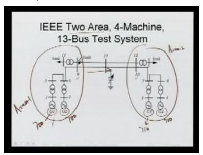
To understand this, how we are going for the multi machine system, we will see the I e e e system, that is a 2 area system - here this is a area 1, this is your area 2; where the 2 machines in this area, generator 1 and generator 2; in this area 2, we are having generator 3 and generator 4. So, this is your nothing but area 2. Here, I am calling this is area 1.
