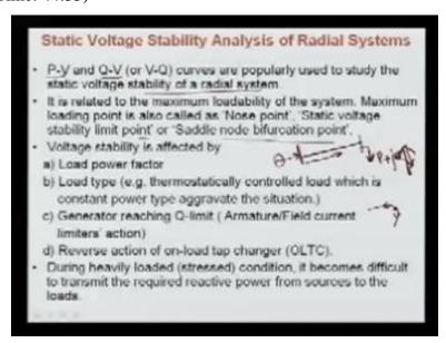
So, the static voltage stability analysis of radial system, here what we do? Normally we use the P-V curve, is very properly used, P-V and the Q-V curves are popularly used to study the static voltage stability of the radial system. Radial system, you know, radial system here your system which is feeding power here, that is coming from some system, then it is a line, and then we have here load. So, this is called radial system.
