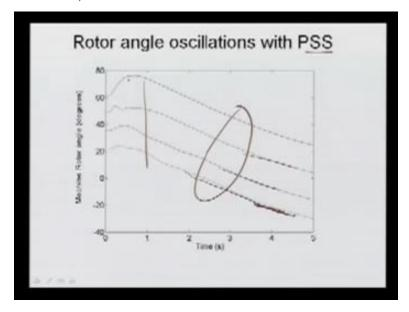
Using this, here what we did, again we did for the same fault and then we measure the rotor angle oscillation of power system stabilizer with the stabilizer here. Now you can see the delta. Now, it is again in the narrow band and then you can say, the delta is here decreasing and now it is going to be steady state. What does it mean? If you are taking one as a reference here, all the 4 generators we are measuring.
