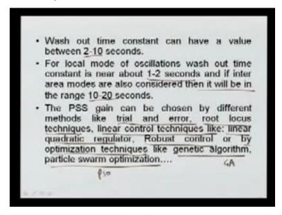
Now, here the washout time constant can be value between this. Here, in the power system stabilizers, you can see here, just we have used here, this is a washout time constant T w, and also we require the terminal voltage here the T r. So, the time constant here can be taken as here, already I have explained here. The washout time constant can have a value between 2 to 10 second.
