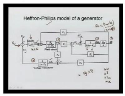
After tuning just we have to use those incomplete system dynamics and then we have to see the performance of the system. To go for the detail model of the power generators the Heffron-Philips model is very popularly used. And, it is here just we have represented; you can see this is your Philips, Heffron-Philips model of a generator. This model is suggesting the 9 states of this generator model completely.
