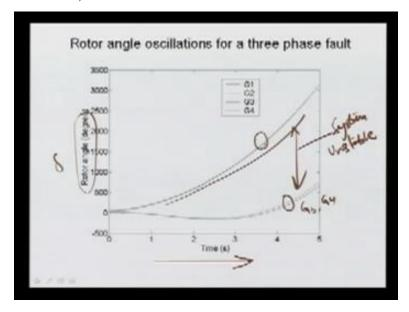
Now, we can also see the performance that is a rotor angle oscillations for a 3 phase fault. We apply the 3 phase fault, you can see here; you can see here, sorry. So, this is you can say apply the 3 phase fault, here this is your 3 phase fault. Once we are applying then the system performance means how this machine dynamic, how this delta of these machine are changing along again, and again the delta as well as the speed we have plotted together.
