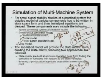
So, if we are going to simulate your small signal stability in the large power system or you can say multi machine system where number of generators are more, then that can be analyzed to consider the dynamics of complex system. For a small signal stability studies of a practical system the detailed model of various components has to be written in state space form and then linearized equations are derived.
