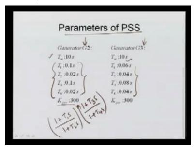
Now, the parameters here, the PSS parameters, that has been used. And, we are using at PSS generator 3 and generator 4 because generator 1 and generator 2 they are very much close together, they are synchronizing at one bus. Here, generator 3 and generator 4 are together. So, we have taken the washout filter time constant T w is the 10 second, this is also 10 second. These are basically your the time constant for the power system stabilizer, once again I said.
