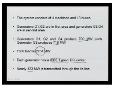
The system consist of 4 machines, as you see, the G 1, G 2, G 3, G 4, and it is having 13 buses. Generators 1 and 2 are in the area 1; generators 3 and 4 are in area 2. Generators G 1, G 2 and G 4 produce 700 megawatt. However, your generator 3 is providing this 716 megawatt. Means here, your this generator 3 is giving 716 and others are feeding the 700 megawatt; means, here is a 700, this is your 700; this is also producing 700 megawatt.
