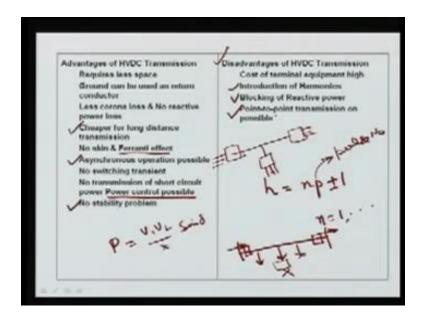
The various advantages of HVDC transmission system that it requires less space; less space in terms that we have normally the two wire system. We may have the homopolar operation; we may have the bipolar operation; we may have the monopolar operation. So, only we require the two conductor's maximum in the DC system, and also here there is no compensating devices required, although, we require the converter stations as well. So, in over all the DC stations are they require less space.
