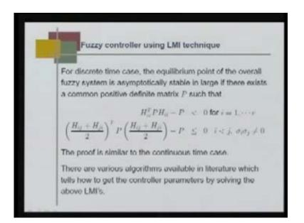
Similarly, for a discrete time case, we can follow the same method. The linear matrix inequality equations would look like this:  $H_{ii}$  transpose P  $H_{ii}$  minus P less than 0, and this quantity is less than or equal to 0. This gives you an idea of how the T-S fuzzy model based controller can be designed using LMI.
