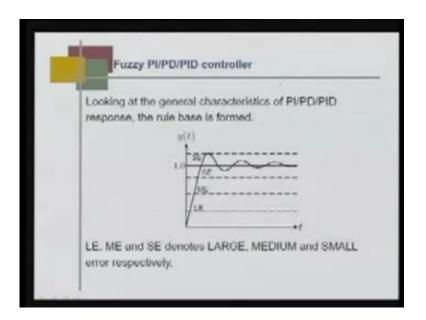
Now let us look at the fuzzy PI/PD/PID controller and how it would behave when the normal rule base is formed. This shows the general characteristics of a response of a system, given a step command. The system is at the origin and we give a step command – unity step command 1. Then, we would like our system to behave like this. What we would like to see is whether we can now guess our rules such that our system would follow a behavior of this kind.
