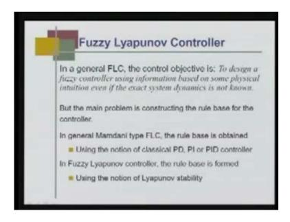
In a general fuzzy logic controller, the control objective is to design a fuzzy controller using information based on some physical intuition even if the exact system dynamics are not known, but the main problem is constructing the rule base for the controller. In general, Mamdani type of
