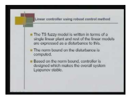
Now, we go to the linear controller using robust control method. In this, the T-S fuzzy model is written in terms of single linear plant and the rest of the linear models are expressed as a disturbance to this. The norm bound on the disturbance is computed. Based on the norm bound, the controller is designed, which makes the overall system Lyapunov stable.
