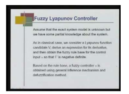
Fuzzy Lyapunov controller: assume that the exact system model is unknown, but we have some partial knowledge about the system. Then as in classical case, we consider a Lyapunov function candidate V, derive an expression for its derivative, and then obtain the fuzzy rule base for the control input u so that V dot is negative definite. Everything is qualitative; I will just show you how it is.
