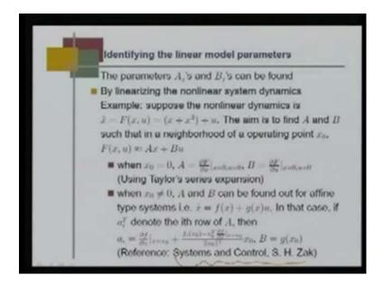
Once we understood what the T-S fuzzy model is, the next step is to derive the T-S fuzzy model. We can derive the T-S fuzzy model by direct system identification or by linearization of an actual nonlinear plant. I will just explain to you, how we linearize a plant.
