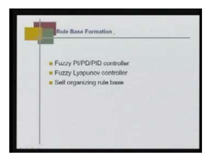
As I said, the rule base formation can be done in three types. One is using the idea of PI/PD/PID controller response – the generic idea that we have of how the normal response of a PI/PD/PID controller would look like. Another analysis is the Fuzzy Lyapunov concept – Fuzzy Lyapunov controller concept. Here, the rule base is formed using stability notion and the self-organizing rule base, where all the parameters of the fuzzy logic controller are generated using the optimization concept.
