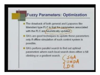
Normally, the first case is heuristically updated. We take the help of heuristics – some kind of a trial and error method. Nowadays, the normal practice has been genetic algorithms or evolutionary computation. What are the GAs? The genetic algorithms perform parallel search to find out optimal parameters, where each local search does either a hill climbing or a gradient search.
