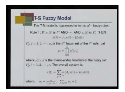
What does it mean? I have the i th rule as I said earlier. If  $x_1$  t is  $F_1$  i and so on and  $x_n$  t is  $f_n$  i, then x dot t is  $A_i$  x t plus  $B_i$  u t and mu<sub>i</sub> is the associated membership function with the i th rule. Then, we saw that the overall fuzzy dynamics x dot t is sigma<sub>j</sub>  $A_j$  x t plus  $B_j$  u t, where sigma j is defined like this.
