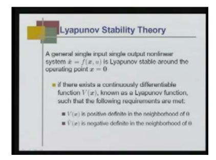
What is Lyapunov stability? The Lyapunov stability is: A general single input single output nonlinear system x dot f x, u is Lyapunov stable around the operating point x equal to 0, if there exists a continuously differentiable function V x known as a Lyapunov function, such that the following requirements are met: V x is positive definite in the neighborhood of the origin and V dot x, the rate derivative of the Lyapunov function, is negative definite in the neighborhood of the origin.
