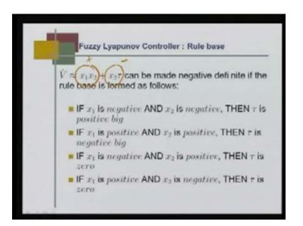
The second rule is  $x_1$  is positive and  $x_2$  is positive. That means this quantity (Refer Slide Time: 20:09) is again positive and this quantity has to be negative now, because, this is positive. To make it negative,  $x_2$  is already positive, so tau has to be negative. Then tau is negative big.
