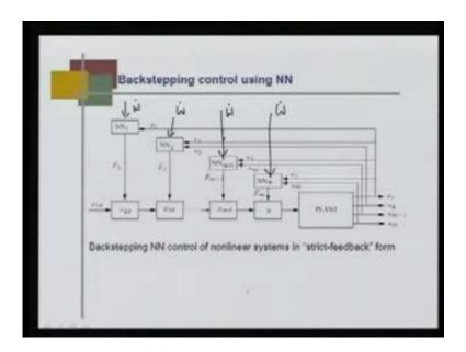
This is your back stepping controller. We design what is u and u utilizes the neural network  $NN_m$  whose output is  $F_m$  hat. Also it utilizes  $x_{md}$ , the information that is given by back stepping approach, because given  $x_{1d}$  I find out, what must be  $x_{2d}$ ? This is my first  $F_1$  is approximated by neural network 1, whose input is only  $x_1$ .
