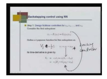
The back stepping control using neural network; this is the theme of this particular class today. So, I introduce, what is back stepping control? Now, we will go in detail design using neural network. Design a fictitious controller for  $x_2 x_3$  and  $x_m$  is a first step. Consider the first subsystem in strict feedback form, that is,  $x_1$  dot is  $F_1 x_1$  plus  $G_1 x_1$  into  $x_2$ .
