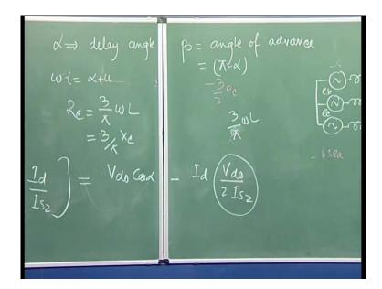
So, we have a two terms now, in the inverter operation which normally define one is called the angle of advance. You know alpha, here it is delay angle normally it is called. And your beta is your called angle of advance, advance angle is also true and it has relation because this your beta is nothing but your pi minus alpha.
