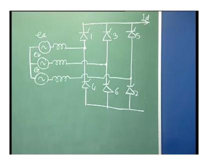
Last time our last lecture, lecture number 5 I explained about how to calculate the dc output voltage of the circuit when effect of this inductances are taken care. Means we are having the u is less than thirty degree u is less than 60 degree sorry.
