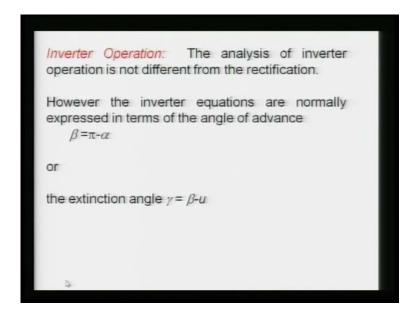
Now let us see the difference in the converter and inversion operation is not big. It is here the analysis is almost same only this your advance angle, it means alpha that is a delay angle is more than 90 degree.
