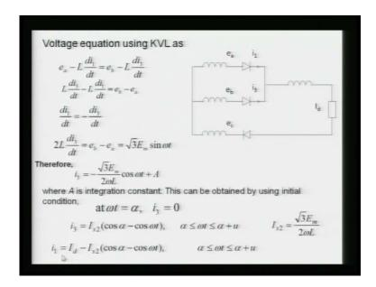
Now, we have to see what will be the pattern of current that is going to be taken care by here because earlier it was I d once 3 was fired then current is shifting from here to here. And this valve 3 is taking complete current just after the commutation period so here it was before this it was I d in the valve 1. And once during the overlap period the current
