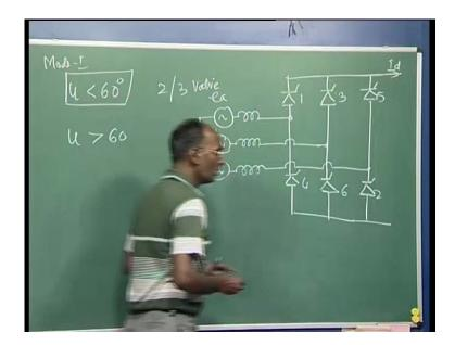
So, u is less than 60 degree and another mode we will see u is more than 60 degrees, but right now I am consulting this. Here thus called mode 1 and again I can say 2 and 3 valves conduction is the pattern. So, one straight forward that we can go for the 60 degree pulse the output voltage we saw and then we can take the average out for that 60 degree and that will be the DC output voltage.
