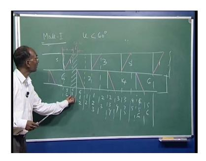
So, on and the conduction of each here it was your 120 degree. This 120 degree here this each valve in the, it is conducting for 120 degree. However, the pairs were conducting are the 60 degree.
