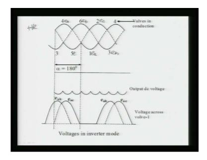
To know the inverter operation again the circuit which I had shown here this is 6 pulse rectify with the numbering of valve 1 3 5 and 4 6 2 we have the 2 groups.
