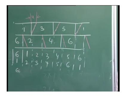
You can see here, if I can draw the upper valves number here. Upper valve is your 1 3 here 5 then again it will be 1. The lower valve here, I can write here, lower valve here always it will be the mid of this. So, this is your 2 here 6 here your 4 here again 6 and again here we are getting the same 2 and etcetera.
