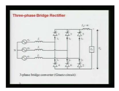
In this case, here your valve here one is conducting for 120 degree and then it is coming here may be your one and two is conducting here this is coming. And again you will find sometimes one is also conducting means this phase current here will be one 120 here
