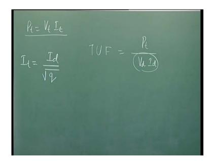
The Pt is nothing but your the secondary side here your r m s a c r m s divided by the your DC power. To calculate what will be the Pt? This is very clear in any output of the converter circuit, it is the V d that is a output the DC voltage and I d is the DC current and we have assume this DC a current is constant in the your DC link.
