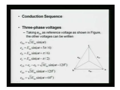
Now, here let us see the conduction sequence conduction sequence as I said the name the numbers of the valves are given in a such a way that you can very easily recognize.
