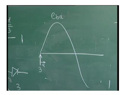
Now, this is your let suppose, here it is e b a I am taking as a reference. Means here this will be the instant when the valve 3 can be fired. Because this is a commutation voltage means you can fire at this instant or even though after delay of any angle alpha this valve can be fired because before that 1 and 2 were conducting. So, 3 can only ignite I from this position to up to this position.
