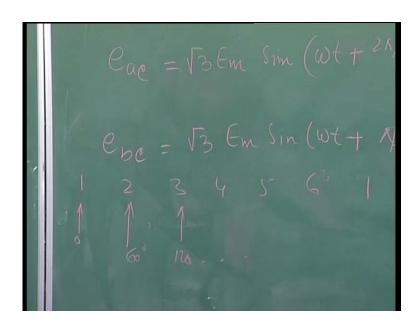
Means here, your let suppose here valve 1 2 3 4 5 6 and it is one again. So, if we are giving here at the 0 instant here this valve is going to be given you are taking this as a 0 axis, then this valve is going to get a pulse after 60 degree. Similarly, here now it is going to be 120 degree and so on so forth. And it is a equal intervals here we are giving the pulses. The reason here we are assuming the symmetrical conduction pattern that is
