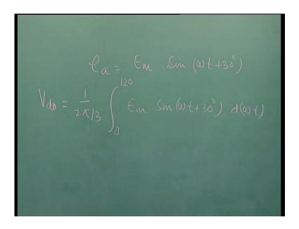
Now we can write this e a is... it is nothing but your e a here; it is your e m; E m it is your peak value of the phase voltage and then here I can write sine omega t plus thirty, because it is a 30 degree shift. You can see here, this is the going be e a going to be zero at this point means, this angle is your thirty degree.
