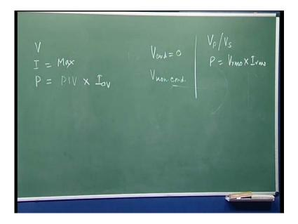
Normally, we say that the thyristor or valve rating if your voltage current and it is a power rating here this voltage rating is nothing but it is the peak inverse rating, peak inverse voltage that is appearing across the valve this power is nothing but it is your the
