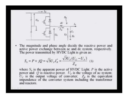
So, this is you can see, this is the current which is flowing from here, we are having this is this inverter operation, we are having single phase is represented by you can say I d is flowing and thus we are having our I g, it is your based technology. And this is the voltage that is from 0 to this U d and I can say, this is your inductor which is connected
