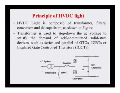
Now, we will go for this principle of HVDC light, so the principle of HVDC light that can be understood by this diagram, you can say the HVDC voltage source convertor is basically composed of whole transmission. Basically, I am talking is composed of transformer, you can see this is a transformer, this is a convertor transformer we call it that is connecting you are AC system, then with the convertor system, we are having the filters, we also need the filters.
