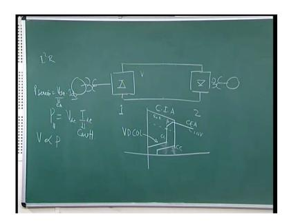
Now for example, you can see here the rectifier is operating on constant current; however, this is operating on CEA volt or vice versa. If the voltage is reduced,
