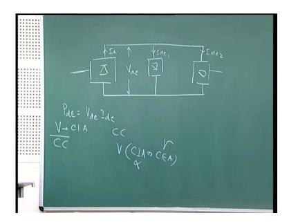
So, you have to add the DC equation for this, another some extra governing equations that should be used in the DC part and then finally, you have to form AC DC equation, whether you are going for the sequential or you are going for the elimination variable method or unified methods, then you have to eliminate those variables and you have to solve, and then you can go for the load flow.
