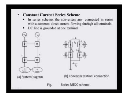
So, this is the series multi-terminal DC schemes. To combine with, we can say parallel here MTDC bipolar scheme with the mesh DC network.
