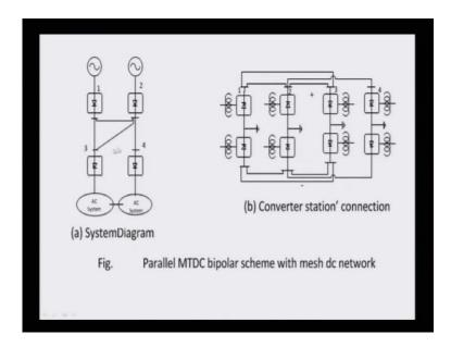
The previous was radial. Here you can see, this is your DC terminal converter station 1, this is 2, this is 3 this is 4, but here you can see the network here, it is the mesh network, it is not radial; however, in the previous case, you can say it is a radial. It is coming and going here, so this is almost radial. So, this is a radial DC network; however, we can find here it is we are having a mesh network and the connection in this.
