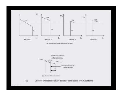
Now, what you can see, once you are operating here, so, your... This is a characteristic of this, so, it is operating on CIA, and others are operating in the constant current control here (()) oh sorry, here this is operating on CC and CC and this is also operating on the CC. So, this is operating on the constant current and this is the overall characteristics and then control characteristics of the parallel connected multi-terminal DC systems.
