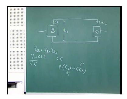
If sum of the rectifier voltage at the ordered current is greater than the sum of the inverter voltage, then the rectifier with the lowest current order assumes the current control, otherwise the inverter with the higher voltage, higher current order assumes current control. Basically this a philosophy that which one will be the constant current control; suppose you are having the variety of converters, then who will be taking this. Already I said here, the rectifier will be taking.
