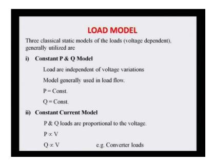
So, with this, we have this governing model and and now we have to go for, this is a load modelling. So, let us start the load modelling as I said is a fourth component that is a load should be also model accordingly, depending upon the need. In the classical normally, the loads are classical analysis of the transient stability, the loads are fixed but, if you are going for the detailed analysis of the transient stability then you can model the load accordingly.
