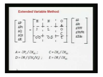
In that we were calculating the various elements of the Jacobean, you can see the extended variable method, because we are extending the DC variables here, the X d c and we are having the corresponding column and the row and the three equations R 1, R 2 and R 3 those are corresponding to three basic HVDC equations. So, also we saw the total X d c is seven variables and out of that we have to specify the four variables and
