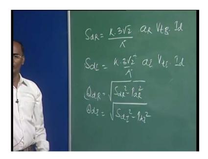
Similarly, we wrote for here S d I it is K 3 under root 2 over pi a V t I into I d we have this we have the P here P d R and the P d I now we have to calculate the Q d R and Q d I. So your Q d R we have to write a function now we are getting this function because this is your one of the variable this t is here it is coming in the AC so we are is not taking care here because other elements have already taken care of this and I d in this case is also constant.
