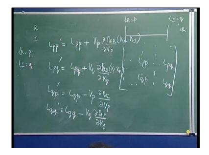
Now, let us see this L, as I said only we are going to modify the corresponding to R that is, rectifier and the inverter, so the corresponding to the p, we are going to write, L p p, why I am writing the p, I am writing this terminal t R, is as a p, otherwise we can write t R, t R because what is the name of this bus, this is terminal R, this is your terminal I, it is q here, it is p, it is easy to just denote.
