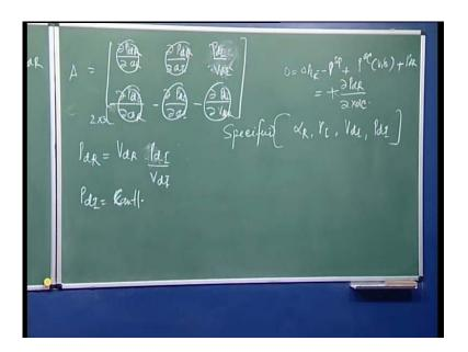
If you are calculating this A and C because in A and C, it is not R 1 R 2 R 3 see this matrix here, this a is corresponding to your real power of the terminals of the HVDC derivative of X d c means, I can say a already even though we have defined also in this, I can write this will be 2 cross 3 matrix, because the P the t R and the t I are the 2 rows here so I can write del P t R del whatever in this case your X 1 and this is your a R
