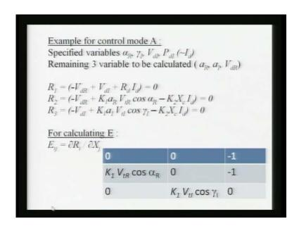
And in the last turn, we were calculating and we found that this matrix, we decided to calculate e I j means, we saw for one example that is your control mode a, where we are having the specified variables your alpha R that is a rectifier delay here the extinction angle of inverter and the V d I is the inverter voltage and the power at the inverter end.
