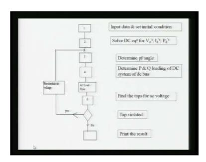
As I said in the sequential load flow methods, we solve first a c then we go for D C AC DC and D C always AC DC AC DC AC DC and finally, we will get the conversions. But, it is not so simple like A C D C you have to see we require something we have to calculate the something stopping criteria.
