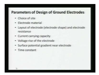
Now, let us see the parameters of what we of the ground electrodes where you are going to put? We saw the characteristic required for the electrodes it should be cheap another
