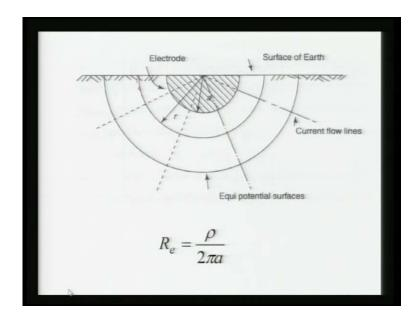
Now, let us see how to calculate the grounding resistance, the grounding resistance here let us suppose, we have a hemisphere conductor half of this it is on the ground this is a conductor we will see once it will go down also later on. But here to see this is your conductor of having hemisphere this and it is radius is a resistance will be this much. How to proof it? We can just calculate this current density the current, which is flowing
