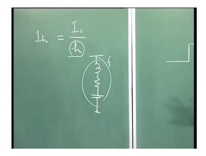
Now, to to filter out because, we saw your harmonics component here, it is basically if it is a fundamental component, then it is your h is harmonics; so, your highest current in A C side, it will be the fundamental component divided by that harmonics component. And now, you can see if it is this h is low this value is larger; and if it is h is higher this component value is very less. So, we should not worry about that, it can be allowed to enter into A C system.
