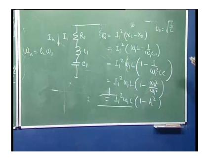
Let us, suppose the current which is flowing here it is your I this I 1 I am talking for the fundamental component and I h for which it is designed here which is flowing it is designed for that tuning. Because, it is having so many components, it is current is flowing, because it is offering the impedance for all these components I 1, I 2, I 3 whatever although it is 0, I 2, so I 5, I 7, I 11 or something all the component.
