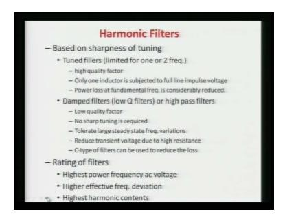
Another is based on your sharpness of tuning and you know there is a two type of filters are classified in this, one is called the tuned filters. Tuned filters, normally it is limited for 1 and 2 means you can go for single tune filters, we can go for the double tune filters. And another is your damped filter or sometimes called the high pass high pass filters.
