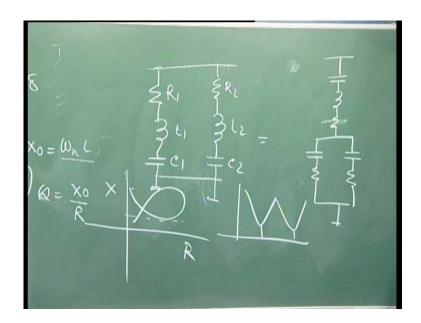
Like here, we are having your resistance, here your inductance and this is your capacitance, here ground I can say it is R 1, L 1 and C 1 this is tuned for one frequency; and if you are having another impedance here, resistance here, capacitance here I can say R 2, L 2, C if they are connected here the parallel here, then we can say it is a double tuned filter.
