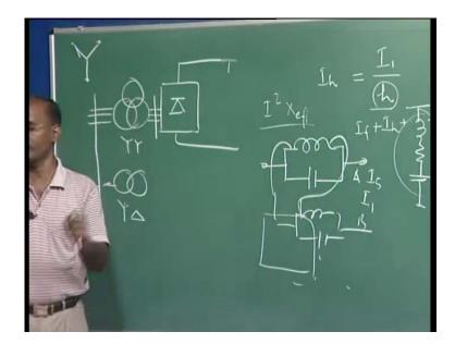
Series type as usual, here this is your inductor, this will be your capacitor and this is put in the line. So, if you are puttying here this is your series, this side also you can put here in the each lines, these filters what happens? They basically provide if any harmonic component entering here, the combination will provide the infinite path it will just behave like a open circuit. So, it will not enter to your A C system.
