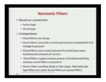
Now, another criterion is based on the type of connection. Here, every time I am showing this is just like a shunt. So, based on the connection we can say our filters can be categorized or you can you can say classified into the two types, one is your series type and another is your shunt type.
