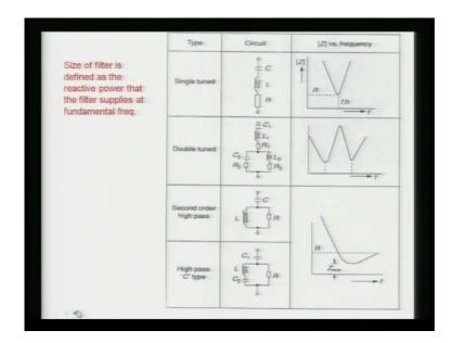
Let us see the, what is the C type and what is the configuration of this? You can see here, this is as I said, here it is your single tuned r l c filter here and you can say, it is tuned for particular frequency, one frequency where it is offering the minimum impedance that is the resistance r. And so this is a r l c series circuit.
