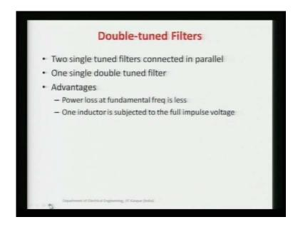
And we will see the various advantage here the two tuned filters as I said, they are connected in the parallel, so this is here. And we are having the single double tuned filters here. The major advantage here in this the loss is minimum. And also, here one inductor is subjected to your full voltage.
