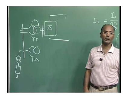
So, your H V D C system it will again this is your converter transformer, this is your A C system, we are having here rectifier, this is your link. So, if your filters are A C side, it is called A C filters; if you are using the filter the D C side, it is called the D C filters as usual. So, A C side basically we use the primary side of here. Now, the question is we can use, this is your three phase going, we can use the filter here, we can use the filter here.
