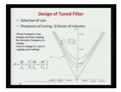
In this tuned filter design, what we do? We want the, what will be the size, and what will be the softness of the tuning, that is basically related with the quality factor of inductor. So, here I have written the few things here what is the changing the power frequency may change. And also, we can change L and C here due to the ageing and heating effect; to analyze this, let us consider the singer order tuned filter that is your r l c filter here.
