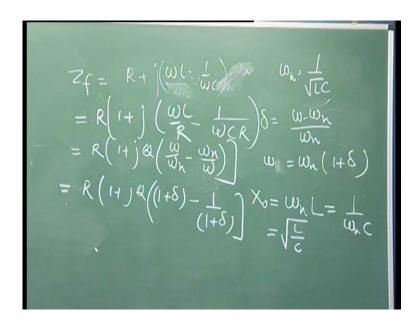
So, this value here will be equal to your under root L C as usual. Another term that is here, delta it is called the frequency derivation term, it is basically defined as omega minus omega n here divided by your omega n. This is also known as the d tuning factor or it is a deviation of frequency from the tuned frequency, this is your tune frequency.
