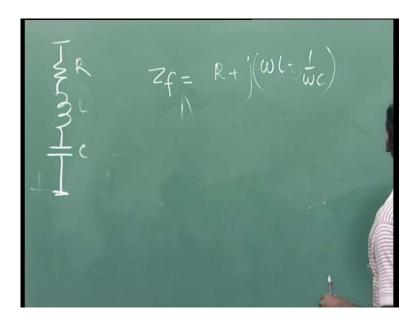
So, we are considering here this is your r and c here, this is a shunt filter, this is your resistance, here your l and c. So, total impendence at any frequency z f can be written
