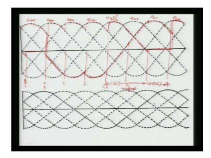
Let us, see and draw the voltage this is as our usual diagrams line to line voltage and here if I can say our e b a is your commutation voltage of valve 3 and now I am talking for the rectifier end similarly, we can talk about the inverter end misfire condition here, I am just discussing the rectifier because is very simple inverter you have to delay again; and then you have to measure from this side rather than this side alpha.
