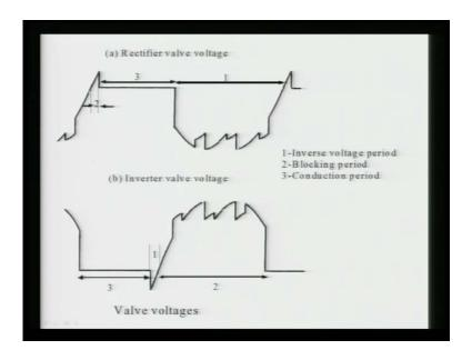
You can say this is the valve voltage across rectifier operation. Because the most of the time in the rectifier operation the voltage across, the valve are either 0 or it is a highly negative and the very small portion you can see very small portion it is a positive.
