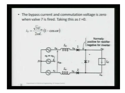
To derive this, you just see this circuit what is happening? As I said 1 and 2 are conducting and at this when e c a is going to be positive, we are giving the pulse to this. Now, I am just writing the equation for this; now before that here I said the voltage will be e b I said this voltage here this is nothing, but half e b; this is minus e b by 2. You can also see from this figure, this is just reverse here and half of the magnitude, this is completely its half.
