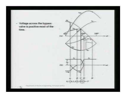
Now, this is very simple in case of rectifier side because this voltage is experiencing negative almost all the time why? Because this voltage is positive; this is negative. So, this valve is experiencing the across this I am talking this minus this is most of the time it is negative, but the reverse is true in the inverter, most of the time this valve is getting the positive already and that is why, here the commutation is very fast and you can commute very quickly without delaying it here.
