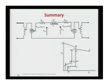
So, this is basically complete energization of these bridges in HVDC link and since, this is the end of this module, now let me summarize what I did in the five lectures. In the beginning, we just develop the equal end circuit, here your rectifier is replaced by variable voltage dc source with the commutation resistance and this is your line resistance; dc resistance basically and this is your inverter side, it can be represented in terms of beta here, it can be also represented in the gamma.
