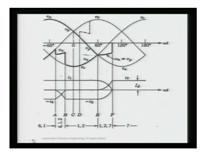
Now, in this first I am going to talk about the de-energization; in the de-energization I said there are two possibilities that either we are having a bypass valve or we can use a pair of valve in the same name and we can make it short circuit.
