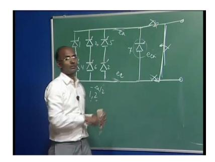
For example here, if this is your 6 pulse converter; this is a all the 6 valves here and we can have a here one option that we can have one bypass, this is called bypass valve. Here is 1 3 5 4 6 2 and this is treated as 7. So, all these are basically the rectifier or g t 0 is switches control switches, I can say.
