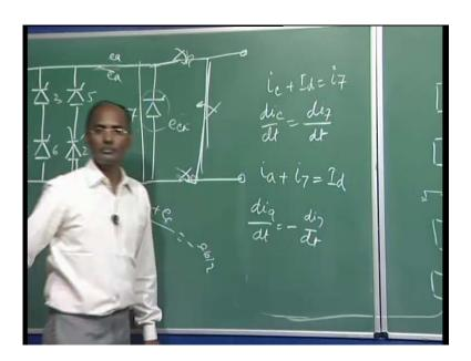
So, this is i c plus I d will be your I 7 means you are here, i c plus I d is equal to your i 7 means if you are differentiating here d i c by d t will be your d i 7 by d t. Here the scenario is different because this current plus this current will be your Id means, your i a plus your i 7 is equal to your I d means I can write d i a by d t will be minus d i 7 by d t because this is a DC current so derivative will be 0.
