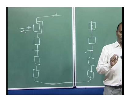
Here, I am talking if you are having let suppose this is one bridge here in one bridge in the one pole here, then one you can take it out and then for that, you know we have to sort this bridge, so that current can bypassed and this is the procedure which I am talking here, the de-energization of this bridge means we are de-energizing this, because we are bypassing here the current completely, and then we can reduce the voltage and we can take it out.
