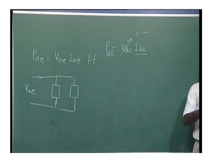
As you know, this power control here this in the DC system, we have the P the dc is nothing but your V dc into your I DC now, this P dc can be controlled by either voltage or by control controlling current or by controlling both but normally what we do we? (()) in HVDC system current is normally kept constant and the voltage varies. It is just reverse in AC system in AC system if you are writing the P ac it is your V ac into your, I ac and sum multiplied by the power factor.
