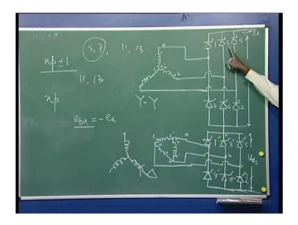
Or you can have this the 2 bridges 6-pulse six-pulse only the difference here the transformer you are using here is a delta delta a star star and here you are using star delta
