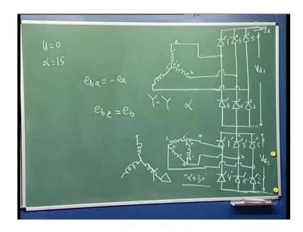
Now, 4 is getting pulse here means commutation is instantaneous we have assumed because u is equal to 0 so, what will happen your which one is conducting 3 and 4 are conducting so, it is e b and a so, it is your output voltage here it is b a so, e b a you see what is e b a e b a it is the negative of this phase so, minus here it is your nothing, but minus e a in this case all these we are talking this case is not with related to this case so, this case is different.
