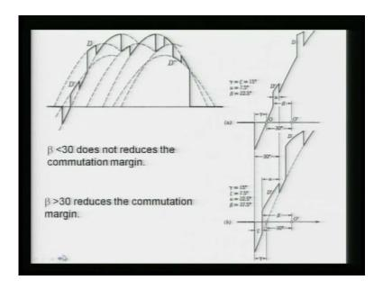
And now, this C D due to this conduction pattern we are having the extra dents here that is, arising for the lower one you see one dent was coming from the top and this was another just deep here it was arising, if the 6-pulses were there now, we are going to add due to that conduction of another effect. We are getting one dent here another here I can say d prime or d double primes are there so, they are going to be added. Now, you can
