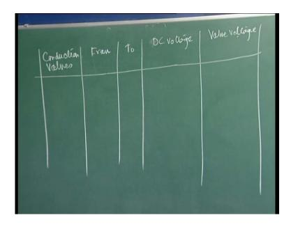
You can write the conduction valves; then you can write the From, To, in angle from then, which angle it will be conducting with period it will from which to which; then, what will be your DC voltage or you can say output DC voltage? Then, if required if you want to draw any valve voltage then you see what will be the valve voltage.
