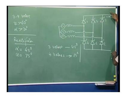
Now, we are here going to discuss again 3 to 4 valve conductions where your u is greater than 60 degree and in this we know alpha should be your greater than these degrees already we proved in the last turn that you must be greater than 30 degree and you're here we are talking about the 3-4 valves conduction mode means your u is greater than 60 degree now, to draw the Rectification operation.
