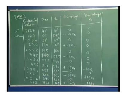
So, here we are starting from 45 degree before that here we are talking the valve 3 is getting pulse. So, this is the case when the valve 3 is getting pulse we are starting from valve 3. So, here now and it will conduct because it is a more than 30 degree. So, here I can say 6 1 2 were conducting earlier.
