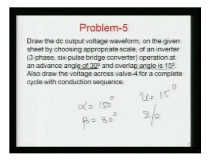
So, let us, draw this DC output voltage for this case, where you are given this your beta is 30 degree and your mu is 15 degree means, you are given alpha equal to 150 degree means, beta is your 30 means, it is this and mu is given your 15 degree means, you are having 2 3 error operation just, you see the angle and you will draw, you will find it is a inverter operation.
