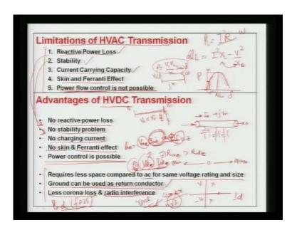
Here, in this you can also see that is I have summarized the 5 major problems limitations are HVAC transmission system that is a reactive power loss the stability concern the current carrying capacity that is the charging skin and the Ferranti effect the power flow control which is not possible in the AC system.
