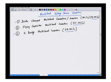
So, these are the three categories that we were discussing in the last lecture, the diode clamped multilevel inverter or DC-MLI or the flying capacitor multilevel inverter if FC-MLI, and H bridge multilevel inverter or HB-MLI. So, in the last lecture, we have already discussed number 1 and number 2, that is we have already discussed the diode clamped multilevel inverter structure, and also we have discussed about the flying
