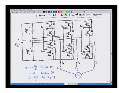
So, we are taking actually a three phase three level diode clamp multilevel inverter, let us first see the structure of this inverter. So, we have three different phases, so let us first draw this complete inverter. So, we have this DC link in this case and let two capacitors here, one capacitor and the other capacity. And then what we have here is that, we have four devices per phase, one this is one leg, second leg, this could be for phase b and then we have the third leg here.
