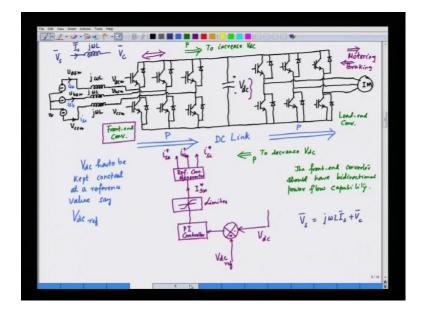
So, we have the structure like this, the front end converter will have a structure in which we have 6 IGBT's, so these gates of the IGBT's the feedback diodes and this converter is
