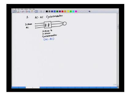
The third possibility we have in this case is a cycloconverter AC to AC cycloconverter, so in this case what we have here, we have the cycloconverter. And the cycloconverter is
