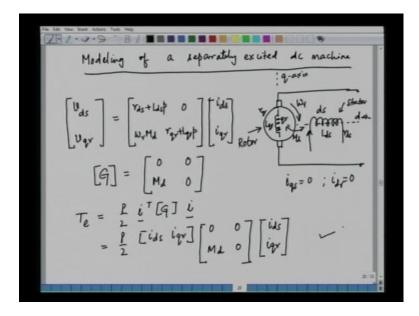
Now, in this lecture, we will try to discuss how this Kron primitive machine model can be used to simulate a DC machine. First of all, we will simulate a separately excited DC machine. Let us see modeling of a separately excited DC machine. Now, what we have here; if you see a separately excited DC machine, we have the armature and we have the field winding. And these are the armature terminals. We can apply some armature voltage here; and this is the field winding.
