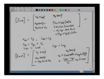
So, let me just we write down the simplified equation of Z actual. Z actual after simplifying, is obtained in the following fashion, which is r d s plus L d s p, M d cos alpha p; p is the derivative operator – d by dt; small p is d by dt; and M d cos alpha p plus M d sine alpha into omega r. Then here we have r d r plus L d r p cos square alpha plus omega r L d r sine alpha cos alpha minus omega r L q r cos alpha sine alpha plus r q
