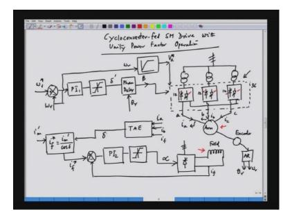
In the block diagram we have the cyclo converter this is the cyclo converter that we have. And cyclo converter is fielding the armature for the synchronous machine this is the armature of the synchronous machine. And the field winding is fed from different
