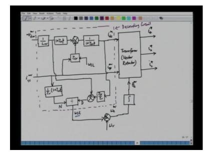
Now, you will see that how we can implement that in case of a block diagram, so we will take an block diagram q, so this can be implemented, so what we have here, we have to use a transformation. This is our transformation block, in which we can feed our i d s m
