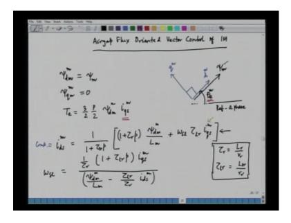
Now, we have already seen that in air gap flux oriented vector control, the d axis of the reference frame is oriented along the air gap flux vector. So, what we do here is the following, that this is the reference axis, reference of phase a of the indexing machine, and let this be the air gap flux vector, and that we symbolized by psi m. And what we do we orient our d axis along the air gap flux vector, this is our d axis, and we call this to be d m and the q axis is right angle to the d axis.
