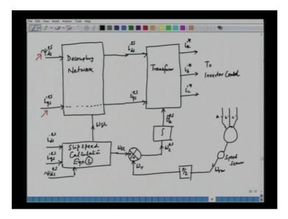
And integration of that will give a the angle of the stator flux vector, and the angle in this case can be use to transform i d s and i q s into i a, i b, i c, which will be impress on to the machine by using the invert. So, this is something similar to that of the air gap flux oriented vector control, and this is also little bit more complex, because you know that we have to use this decoupling network.
