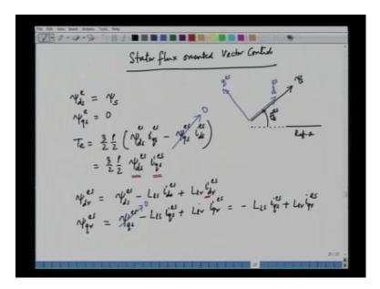
Stator flux oriented vector, now in this case also we can say that, if this is our phase a axis is the reference a and what we are doing here, we are tracking for the stator flux. This our psi s and what we do here we orient our d axis along the stator flux vector, so we can orient our d axis along this, so we call this to be d e s, symbolizing that this is a rotating reference frame, and this is a stator flux reference frame. And the q axis is
