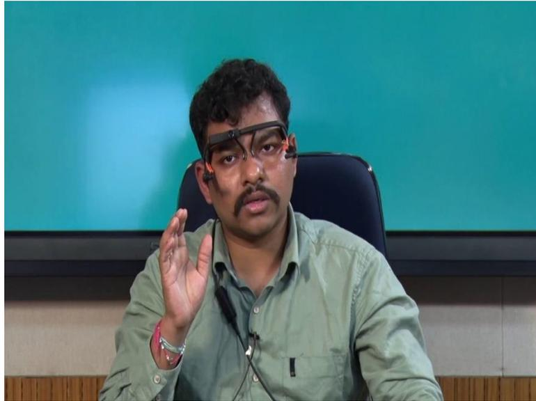
So, first you have to wear the eye tracker and when you wear the eye tracker adjust these pupils, so that it has highest confidence. Confidence is it shows how much of accuracy or how much of pupil is being detected and how much of pupil is not being detected.
