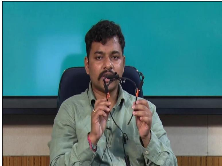
So, today we will move forward by discussing the eye tracking device, this is a head mounted eye tracking device and the maker is Pupil Labs.
