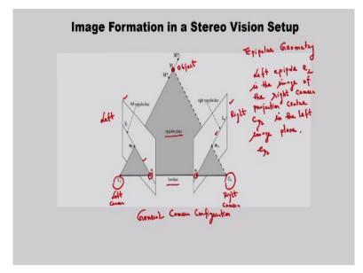
So in this setup I have shown the image formation in a stereo vision setup. So this configuration is called the epipolar geometry this is called the epipolar geometry. So, what is the definition of the epipolar planes? So, here you see I have the left camera projection center, this is the left camera projection center, this is the right camera projection center and corresponding to this two cameras I have the image plane.
