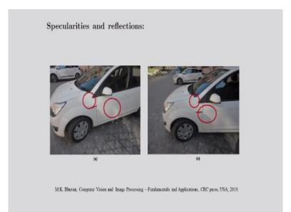
The next point is the specularity and the reflections. So, already I have explained what is the specular reflections? For a specular surface the radiance leaving the surface are dependent on angles. So the disparity map obtained from the stereo image pairs may not give actual information of the specular surfaces. In this example I have given the specular surfaces, this
