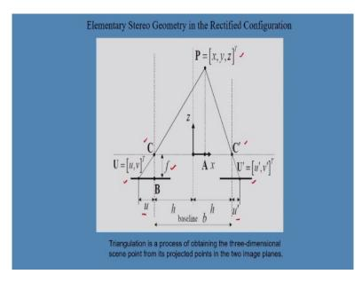
Now, here I have shown the elementary stereo geometry in the rectified configuration. So that means from this configuration I want to determine the depth information. So, let us see this configuration. So in this configuration, I have two cameras the projection center is C and C dash. Here this is the left camera and this is the right camera and this is the point the scene point is P x, y, z the scene point is x, y, z.
