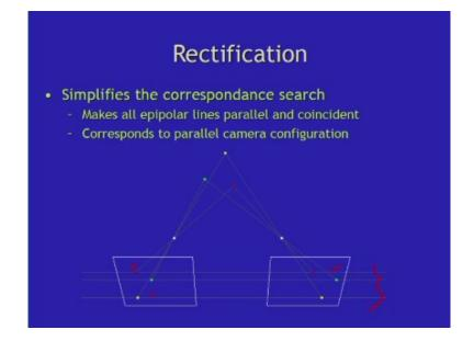
But in this configuration I have shown the epipolar lines are parallel now. So, I am making the epipolar lines parallel and actually this configuration is called the canonical stereo configuration. So, in this case you can see the 2D searching problem is converted into 1D searching problem.
