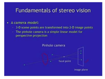
So, here I have shown the image formation concept that I have already explained that is the pinhole camera model that is the very simple model and simple linear model and it
