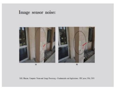
Now let us consider another problem that is the image senor noise because of the noises in the camera you can see this noise is here and noise present in the image then also it is very difficult to find the correspondence between the images. So, one technique we can apply that is the preprocessing of the image that is you can remove noises in the image by filtering.
