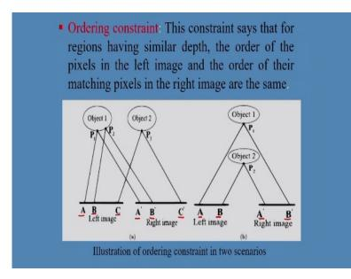
And this is very important the ordering constraints. This constraint says that for regions having similar depth the order of the pixels in the left image and the order of their matching pixels in the right image are the same. So, here I have shown two cases is A and B illustration of ordering constraint in two scenarios. So, in the first example the ordering constraint is fulfill. Why it is fulfill?
