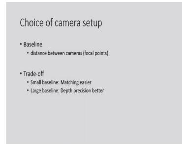
And in this case the choice of camera setup is very important. The baseline is the distance between the camera, the camera means the center of the projections of the camera the left camera and the right camera and if I consider small baseline then in this case the matching will be easier and if I consider large baseline then depth precision will be better.
