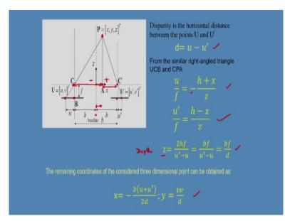
So, same configuration I am showing here. Now, I am defining a term that term is called the disparity. Disparity in the horizontal direction between the points u and u dash that is u minus u dash. So, in this diagram you can see similar right angle triangle. One is this triangle that is the UCB that is one triangle and another triangle is CPA that I am considering the CPA two right angle triangle and corresponding to the point the coordinate is x, y, z.
