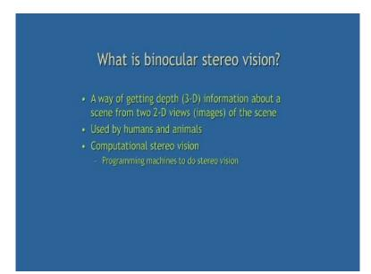
So, let us see what is the stereo vision setup? Now already I told you that image formation process is nothing, but the 3D to 2D transformation. The 3D scene coordinate is transformed into a 2D image coordinates. In case of the human visual system, human brain reconstruct the 3D information. In case of the computer vision we have to develop some algorithm so that computer can determine the depth information. So, for this we can consider a stereo vision setup.
