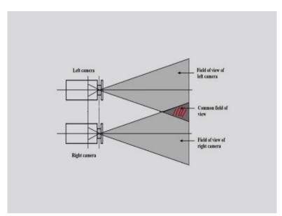
So, in this diagram I have shown the common field of view the two cameras I am considering the left camera and the right camera and I have shown the portion that is the common field of view I have shown.
