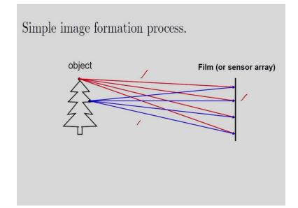
So, I have considered this set up. So, I have considered the object and this is the film. So, in this case I am getting the blurred image because of the intersections of the rays. If you, see the different rays are coming from the objects. And in this case I am getting the blurred image.
