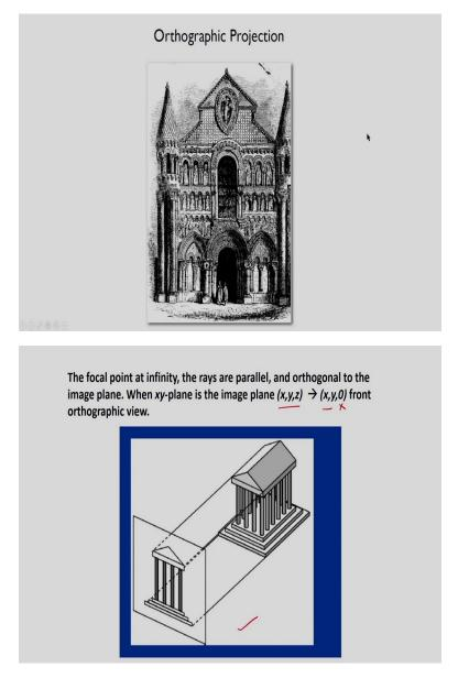
And here I have given two examples. One is the, first one is the perspective projection. And second one is the orthographic projection. And I am shown one image corresponding to orthographic projection. In this case there is no z information because it is mapping from x y z to x comma y.
