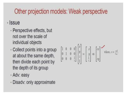
So, the meaning of this, it will give the perspective effect but not over the scale of individual objects. And in this case I had to collect the points into a group that I have shown in previous slide. So, collect the point into group at about same depth and then divide each point by the depth of that group. So, it is the same thing, the scaling of x coordinate and scaling of y coordinate. And this concept, the weak perspective projection approximate the perspective projection.
