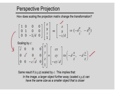
Now let us consider how does scaling the projection matrix change the transformation? So, this is my perspective projection. Now let us consider scaling of x coordinate by c, y coordinate by c and z coordinate by c from the previous equation. Corresponding to this I am getting the same output. What is the output? The output means the image coordinate. The image coordinate will be minus dx divided by z minus dy divided by z.
