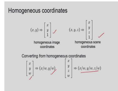
The x comma y I can write in homogenous coordinate like this, x y 1, adding one extra coordinate and if I consider it the scene coordinate x y z, that can be represented in the homogenous coordinate x y z 1. So, I can represent like this. And suppose if I want to convert
