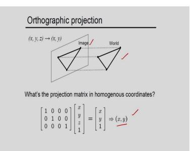
In this diagram also I have shown the same concept. The point x y z is mapped into x comma y. That is the, from world coordinate to the image coordinate I am doing the mapping. And what is the projection matrix in homogenous coordinate? In homogeneous coordinate I can write the, the projection matrix in this form. That is the orthographic projection. So, this is my image coordinate.
