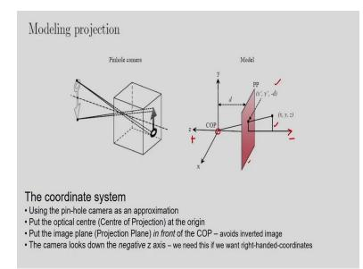
So, here I am shown again the modeling of projection. Again I have shown the pinhole camera model as an approximation. And after this I have shown the projection model. So, in this case I have considered the optical centre that is the centre of projection at the origin. So, COP means the centre of projection and I have considered the object. The object is x y z. And this PP means the plane of projection that is the image plane.
