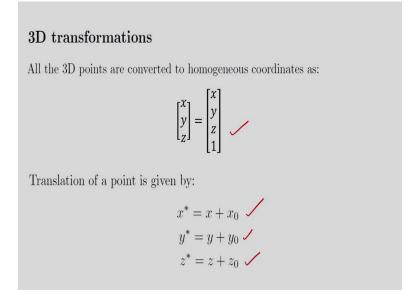
So, next I am considering 3D transformations. So, in the 3D transformation all the 3D points are converted to homogenous coordinate. It is something like this. So, x y z is converted into x y z 1. Translation of the point is given by x',  $x^{i} = x + x_{0}$ . So, the translation along the x direction, translation along the y direction and translation along the z direction.
