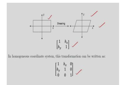
So, here I have shown the example. So, how to do the shearing? So, in this case shearing parallel to x axis I am shown here. So, this is the, suppose object and I have done the shearing. So, this is the matrix for shearing. In homogenous coordinate system this transformation I can write like this. So, the translation operation, the rotation operation, scaling operation and this operation is the shearing operations. The next I have shown one example.
