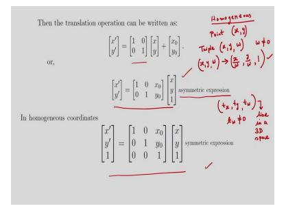
Now translation can be represented like this. So, translation process is  $x'y' = 1 \ 0 \ 0 \ 1$  hat matrix I am considering, into  $x \ y + x_0 \ y_0$ . So, that the previous equation you can write in this form. Or you can write in this form. x'y' is equal to  $1 \ 0 \ 0 \ 1 \ x_0 \ y_0 \ x \ y \ 1$ . So, the previous equation, whatever I have shown in the previous slide, that the translation operation, that operation you can show in the matrix form like this.
