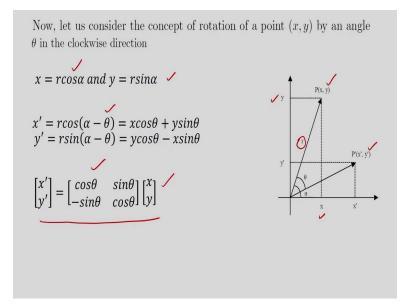
Now let us consider concept of rotation of a point x y by an angle  $\theta$  in the clockwise direction. In this figure I have shown. Suppose the point is P x y and that point is rotated by an angle  $\theta$ . So, what is the new position? The new position is P'x'y'. That point P x y is rotated by an angle  $\theta$  in the clockwise direction.
