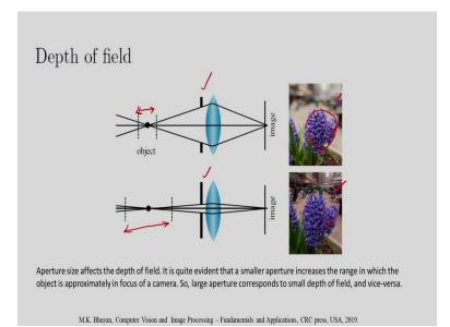
And there is a concept of the depth of field. So, here you see I have shown two cases. In this, in the first case I have shown this portion, suppose if I consider the aperture is wide. And in this case the aperture is narrow. In the first case the aperture is wide, in the second case aperture is narrow. In the first case, only this portion of the object, from this length to this length it is properly focused, the rest of the portion, it is not properly focused.
