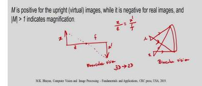
And what is the magnification done by the lens of a camera? The magnification is defined by di divided by d 0. That is the definition of the magnification. M is positive for the virtual image while it is negative for the real image. And if I consider M is greater than 1 that indicates the magnification. So, this is the definition of the magnification done by lens of a camera. So, in case of the monocular setup, monocular vision, suppose this is the object and this is the image.
