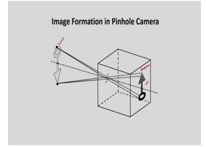
And in this case I have shown the image formation in a pinhole camera. So, this is a very simple camera. So, I have one opening here, small opening, hole is there. And this is my object, and this is the image.
