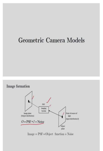
Now after this, I will discuss the concept of the image formation in the camera. So, if you see in my next slide I am going to discuss about the geometric camera models. So, first one is image formation principle. And in my last class I explained about this, what is the output image? The output image is the PSF. And it is convolved with the object function + noise, noise of the imaging system.
