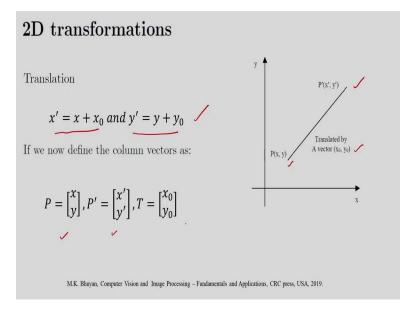
So, first operation is 2D transformations. So, first I will discuss 2D transformation and after this I will discuss 3D transformations. So, first I am considering one point here the point, the point is P, x y. This point P, x y is translated by a vector, the vector I am considering, that is  $x_0 y_0$ . So, it is translated by the amount  $x_0$ ,  $x_0$  unit parallel to x axis,  $y_0$  units parallel to the y-axis.
