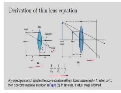
And in this case I have shown the derivation of the thin lens equation. I am considering the convex lens and from the similar triangles, this equation I am getting. What is d 0? d 0 is the distance between the objects and the lens. So, this is d 0 What is di? The distance between the lens and the image. So, I am having the image here. And here I have shown the focal point and also the focal length I have shown. f is the focal length.
