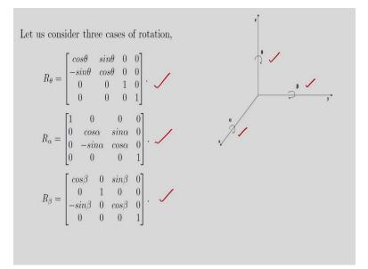
And let us consider the concept of the rotation. Now the three cases of rotations; rotation around x axis, rotation around y axis and rotation around z axis. If I consider rotation around z axis, only x and y coordinates change and z coordinates remains same. Rotation around z axis means it is a
