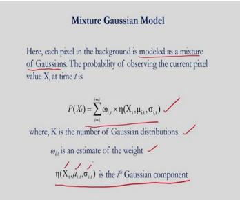
The next one is I can consider the mixture of the Gaussian model that is the Mixture Gaussian Model. So, what is the concept of this? So, each pixel in the background is modelled as a mixture of Gaussians. So, I can consider the pixel as a mixture of Gaussian because a Single
