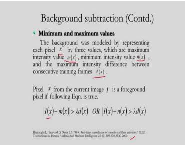
And this is also a very old technique; here it is published here that is IEEE Transactions on Pattern Analysis and Machine Intelligence. So, briefly the concept is like this, so the background is model by representing each pixel, the pixel is x by three values, so 3 values are considered. One is the maximum intensity value m(x), one is the minimum intensity value n(x) and the maximum intensity difference between the two consecutive training frames that is the dx.
