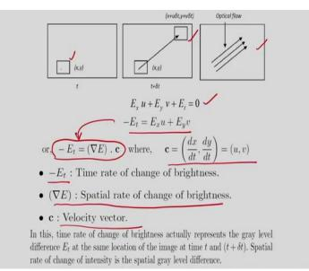
So, the same concept I am showing here, so this path is moving to this position and corresponding to this I will be getting the optical flow. The optical flow it depends on the change of the brightness because of the motion. So, already I have this equation, so this equation I can write like this. So, what is the interpretation of this equation?
