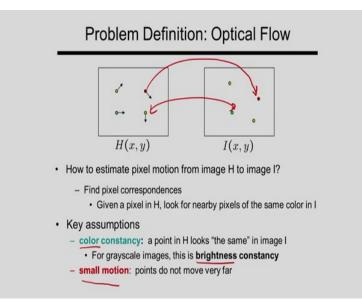
And the problem definition of the optical flow, so here I have shown two images, one is H another one is I. And I have shown some pixels, the red pixels, the green pixels like this I have shown. And the pixels are moving, so I have to determine the motion of the pixels that is nothing but the motion estimation.
