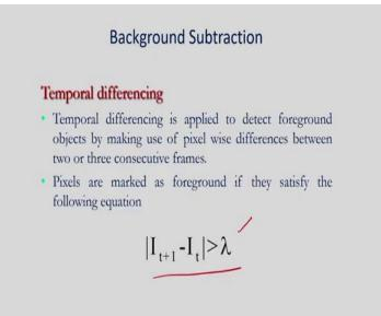
Now I will discuss the concept of the background subtraction. So, one very old algorithm is the temporal differencing. So, this algorithm I can apply to detect foreground objects by making use of pixelwise differences between 2 or 3 consecutive frames of the video. That means I have to find the differences between 2 or 3 consecutive frames.
