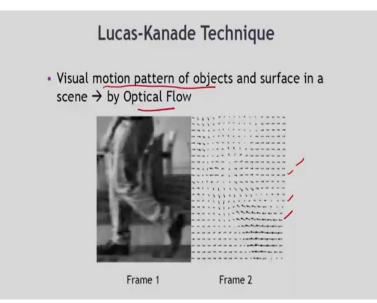
And one important technique is the Lucas- Kanade technique. That is the concept of the optical flow. So, we can determine the visual motion pattern of the moving objects and that is
