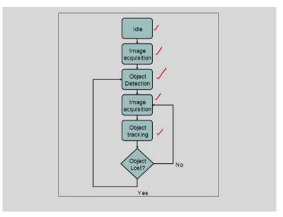
And how to detect the object? That I am showing the simple flowchart here. So, suppose the object is stationary, after this we are considering the image acquisition. After this we can detect object, so object detection algorithms are available. After this again the image acquisition from the video that is the frames I am collecting or the frames I am taking from the video.
