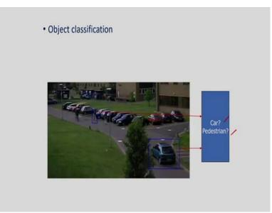
After this object classification, so we can consider the classification of objects present in an image or maybe the video. So, here you can see we are classifying the objects, the car, the pedestrians, like this we can do the classification based on some algorithms. That is also very important. So, we can employ some machine learning algorithms for object classification.
