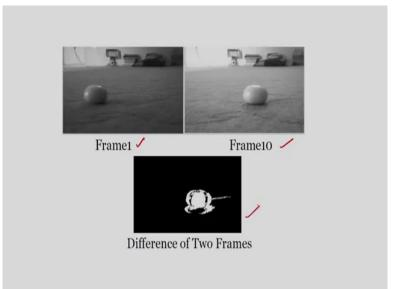
So, again I am showing you the same thing the background subtraction algorithm. So, this is frame one and another one is the fram ten. So, if I do the subtraction, then I will be getting the difference of the two frames that are nothing but the moving objects I can determine.
