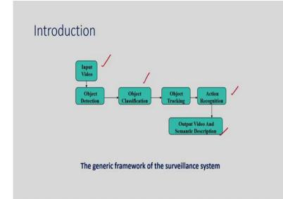
So, let us consider one generic framework of a video surveillance system. So, input is the video. After this we have to detect the objects present in an image, and after this we can employ some machine learning algorithms, the pattern classification algorithms for object classification. After this we can do the tracking, the tracking of the objects, and also we can mploy this one that is the action recognition, that is the activity recognition.
