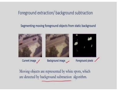
In this case I am showing one example foreground extraction that is the background subtraction that is nothing but the sense detection algorithm. So, this is the current image and I am considering the background image. If I subtract the background image from the current image, I will be getting the foreground pixels. So, this is nothing but the background subtraction algorithm.
