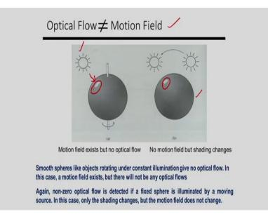
But sometimes, it may not be the optical flow may not be equal to motion field. Here I am giving two example, in the example a, you can see, this object is rotating this is rotating and I have the source, one source is available. So, corresponding to these paths, suppose these paths I am considering, the illumination will be almost constant that means if the illumination is constant then corresponding to this there will not be any optical flow.
