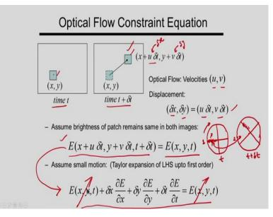
Here I have shown two frames of a video at time t another one is time  $t+\delta t$ . Let us consider a paths at the point x, y. So, these paths I am considering. And other time  $t+\delta t$ , this path moves to this position, second position. So, these paths will be moving suppose. Now what will be the position of the paths in the second image? The position of the paths in the second image  $x+u\delta t$ ,  $y+v\delta t$
