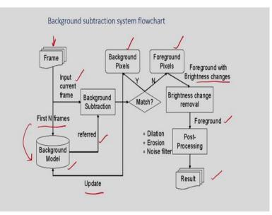
So, in this example, I have shown one algorithm that is a simple algorithm for background subtraction. So, background subtraction system flowchart. So, suppose I have the input video and I am considering the frames of the video. First I am considering the N frames...the first N number of frames I am considering and based on this I am determining the background model. So, the background model is determined from the first N number of frames.
