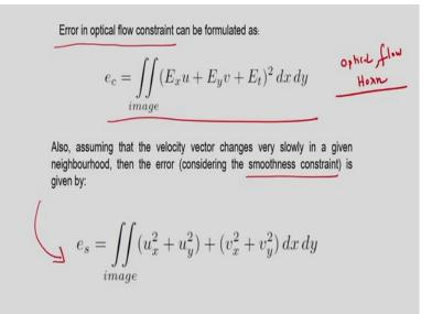
And for optical flow solution, there are many methods, so simply I am showing one method but if you want to see the solution of this method, so you can see the optical flow paper; research paper by Horn, the original paper is by Horn, so you can see this research paper, the optical flow algorithm you can see by Horn, but briefly I have explained the solution of this equation and that is the optical flow equation.
