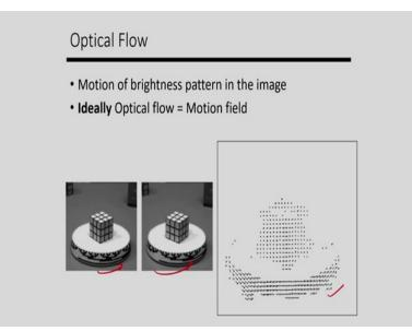
Here you can see in this example I have shown this object is rotating, it is rotating like this in the counterclockwise direction and corresponding to this I will be getting the optical flow that is the motion pattern I will be getting. And ideally, the optical flow is equal to motion field, because the object is also moving and corresponding to this I will be getting the motion factors that is the motion field I will be getting and also the optical flow I will be getting.
