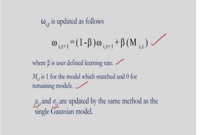
And after this we have to update the weights by using this equation and here the beta is the user defined parameter that is nothing but the learning rate and  $M_{it}$  is 1 for the model which is matched and 0 for the remaining models that is about the  $M_{it}$ . And this mean, mean and the standard deviation or the mean and the variance should be updated like we did in the Single Gaussian Model.
