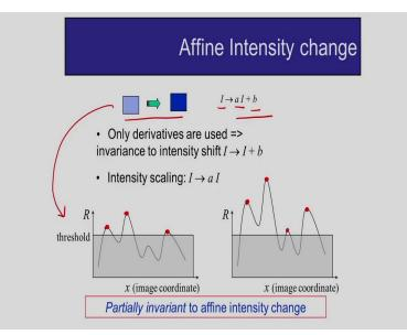
So, in this case I am showing one case that is the affine intensity change. So, I am showing these two images and the intensity is change. So, for this I am considering I is the intensity of the original image and after this I am doing the intensity scaling the intensity scale a into I and I am considering the offset, the offset is supposed to b.
