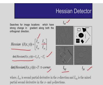
And finally I want to discuss about another detector that is the Hessian detector. So, the concept is very similar, so searches for image locations which have strong changes in gradient along both the orthogonal directions. So, for this also I have to determine the image gradients and I have to determine the Hessian matrix corresponding to the image the image is I x y.
