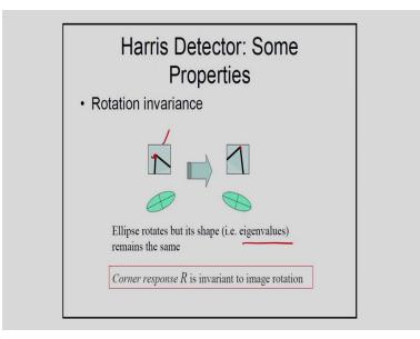
And for a Harris detector some properties I have to explain, the first property is the rotation invariant and in this case you can see one corner I am considering you can see one corner I am considering and it is rotated then in this case the ellipse rotate but its shapes remains the same that means the eigenvalues will remain the same.
