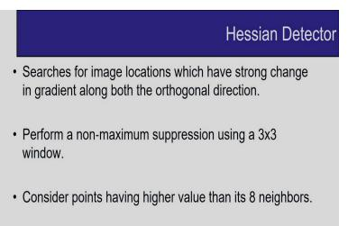
So, in this case searches for image location which have strong change in gradient along both the orthogonal directions and also we have to perform a non-maximum suppression using a 3 by 3 window that is also very important, so I have to perform a non-maximum separation using a 3 by 3 window and also we have to consider points having higher value then it's 8 neighbourhood that is we have to consider and based on this we can eliminate false corner points. So, this is about the Hessian detectors.
