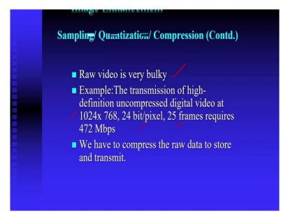
And if you see why we need the compression. Suppose a raw video is very bulky. So suppose in this example, if I considered a digital video, uncompressed video,  $1024 \times 768$  that is the size of the image frame.
