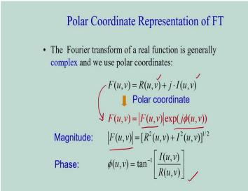
So, already I have explained this concept. If you see F u v, that is the Fourier Transform of an image. If I consider the Fourier Transformation, it has two parts, one is the real part another one is the imaginary part. So, in this case you can see first one is the real part, the next part is the imaginary part.
