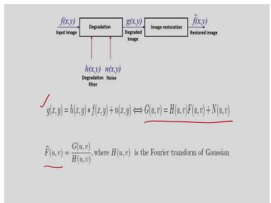
Now, in this case the same thing I am showing here, that is the degradation filter I have shown, the noise I have shown, the input image I have shown, and finally I am getting the restored image. Then in this case this model can be mathematically represented in the spatial domain, and in the frequency domain as follows. In spatial domain I can represent like this the g x y is nothing but h x y, that is the degradation filter, convolution with f x y plus the noise. That is the additive noise.
