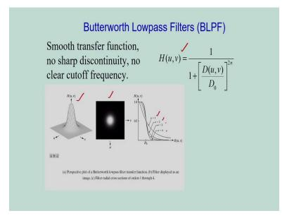
Now, I will consider the concept of the Butterworth low pass filter. And corresponding to the Butterworth low pass filter you can see the function, the transfer function in H u v is equal to 1 divided by 1 plus D u v divided by D naught to the power twice n. And in this case I have shown
