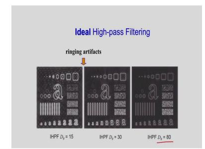
So, in this case you can see the ringing artifacts corresponding to the ideal high pass filter as the transition from the pass band to the stop band is very sharp. So, that is why I have the ringing artifacts. And if you increase the cutoff frequency, the cutoff is D naught, then in this case you can see the ringing artifacts will be less. This ringing artifact concept already I have explained.
