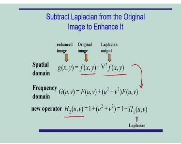
So, how to do the image enhancement by using the Laplacian operator? In spatial domain what you can do suppose I have the original image. The original image is f x y and if I take the Laplacian of the image that means I can select the high frequency component. So, high frequency information is subtracted from the original image, that I am doing.
