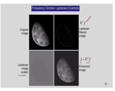
So in this case I am showing one example of the Laplacian, so how to apply the Laplacian of the image. In this case you can see the first one is the original image, the second one is I am considering the Laplacian filtered image. That means I am determining the edges by using the Laplacian. The next one is I am considering the Laplacian image scale, and after this I am subtracting the Laplacian from the original image.
