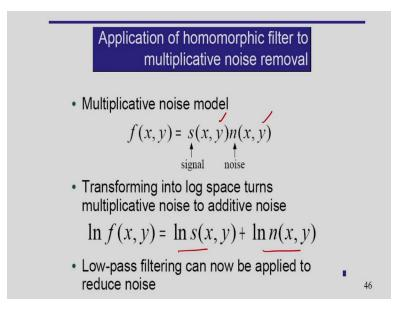
And in this case I can give one example of the Homomorphic filtering to remove multiplicative noise. So, what is this noise model, you can see the multiplicative noise model. I have the signal
