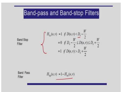
And after this, just I am considering the band stop filter and the band pass filter. And in this case the band stop filter, the transfer function you can represent like this, and again the concept of the cutoff frequency, the cutoff frequency is D naught and W is the width of the band. W is the width of the band. And you can see the band pass filter, what is the band pass filter, 1 minus band stop filter. That is the band pass filter.
