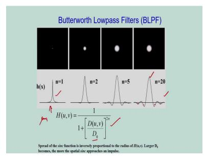
So, in this case you can see I have shown the Butterworth low pass filter that is displayed as an image. So in this case you can see, H u v is the filter transfer function of the Butterworth filter. Now, corresponding to frequency domain, my response in the spatial domain will be sinc function. So, in the case of the Butterworth low pass filter the spread of the sinc function is inversely proportional to the radius of H u v.
