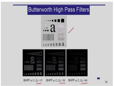
And corresponding to the Butterworth high pass filter, you can see the output, first one is the input image, the next one is the Butterworth filter, order is 2, but D naught is 15. So,
