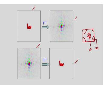
And in this case, I have already explained this one in one of my classes. That is if I take the Fourier Transform of the input image, my input image is this and I am determining the Fourier Transform of the image, so corresponding to this I am getting the Fourier Transform of this. And in this case, if I want to reconstruct the original image, I have to apply the inverse Fourier Transformation.
