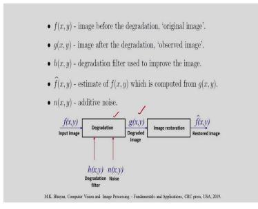
So, the definitions are like this f x y input before the degradation that is the original image. What is g x year? Image after the degradation that is the observed image, h x y that is the degradation
