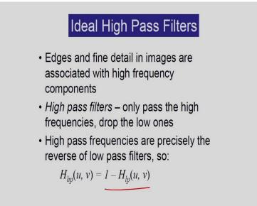
So, for finding the fine details of the image like edges and the boundary I can consider the ideal high pass filter, so high pass filter is nothing but 1 minus low pass filter. So, by using the high pass filter we can see the fine details of the image like the edges in the boundary.
