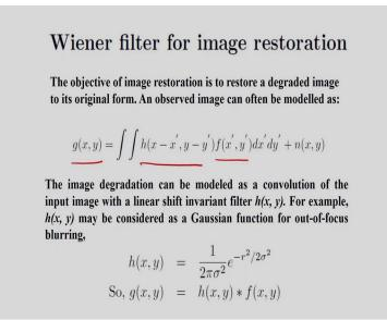
Next, I am considering the Wiener filter for image restoration. This image restoration already I have explained, in this case it is objective, enhancement is subjective. In case of the image restoration model we can develop a mathematical model and based on this mathematical model we can remove the noise or we can improve the visual quality of an image. The objective of the
