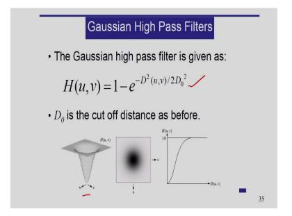
And finally I want to show the Gaussian high pass filter. So, the Gaussian high pass filter is defined like this and D naught is the cutoff distance as discussed earlier. So, corresponding to the Gaussian high pass filter I have the filter function and the filter is displayed as an image and I have the response of the Gaussian high pass filter. Like this.
