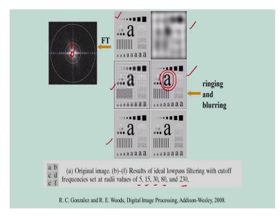
Now, in this case I am showing the example of the ideal low pass filter. And in this case you see my input image is this, the first one is the input image. After this what I am considering? I am considering the ideal low pass filtering with cutoff frequency, that is the cutoff frequency is the D naught and the radii values, something like the 5, 15, 30, 80, and 230. If the radii value is 5, that means I am considering a very small circle, radius value is 5.
