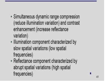
So, already I have explained this concept, the simultaneous dynamic range compression and contrast enhancement. And the illumination component is a low frequency component, that is a slow spatial variation, and a reflectance component is a high frequency information, it is characterized by abrupt spatial variations because it varies quickly at the surface boundaries, edges due to varying phase angles.
