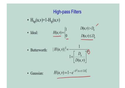
Next one is the concept of the high pass filter. So, what is high pass filter? The high pass filter is nothing but 1 minus low pass filter. So, in spatial domain filtering also I have explained the how to get the high pass filter. High pass filter is nothing but 1 minus low pass filter. So, in this case also I have three cases, one is the ideal high pass filter Butterworth filter and the Gaussian high pass filter.
