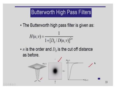
And after this the concept of the Butterworth filter, so you can change the order of the Butterworth filter, n is the order of the Butterworth filter and D naught is the cutoff distance as explained earlier. So, corresponding to this Butterworth filter, you can see the filter function H u v. The filter is displayed as an image and corresponding to this the response of the filter you can see. So, this is the Butterworth high pass filter.
