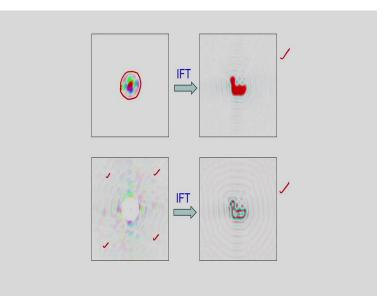
In this example you can see I am considering only the central portion of the Fourier Transformation, that corresponds to the low frequency information. And if I apply the inverse Fourier Transformation, then you can see the reconstructed image. So, this is the reconstructed image.
