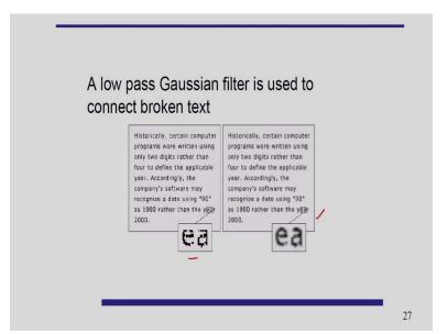
Next I am showing one example, one practical example. A low pass Gaussian filter is used to connect broken text. So, in the first figure if you see, I have shown the broken text here and if I apply the Gaussian filter, the low pass filter, then you can see the output that in this case we can connect the broken text because of the blurring. Because the Gaussian filter produces the blurring of the image. So, that is why the broken text is connected.
