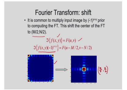
And for the preprocessing what I have to do, if you can see here the Fourier Transform of an image the image is f x y and corresponding to this the Fourier Transform is F u v. So, in this case the input image is multiplied by minus 1 to the power x plus y. Then in this what is the objective of this preprocessing step?
