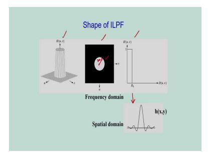
Corresponding to this filter transfer function I am showing the ideal low pass filter. So, if you see the H u v, that is the filter function, that is very similar to the box function. And in the second case I am showing the filter as an image. The filter as an image I am showing. And in the final case, if you see the last case, I am showing the filtered response, that is the low pass filter. And D naught is the cutoff frequency. And already I have explained that D naught is a positive constant.
