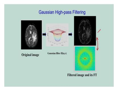
So, here I have shown one example of the Gaussian high pass filter. I have shown the original image after this I am considering the Gaussian filter. Corresponding to the Gaussian filter you can see the output, that is high pass filter. So, I am having the edges. You can see the fine details of the image and corresponding Fourier Transform you can see. Corresponding to this image this is the Fourier Transformation. So, this is the Gaussian high pass filter.
