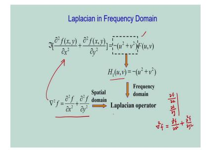
The next one is the Laplacian in frequency domain. This Laplacian I will explain when I will discuss the concept of the edge detection. So, Laplacian is spatial domain is represented like this, that is the second order derivative, f is the image. So, the first order derivative is del f divided by del x. That is the gradient of the image along the x direction and gradient along the y direction. This is the gradient.
