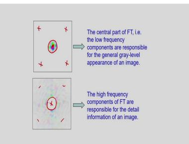
So, here I am explaining this one. The central part of the Fourier Transform, that is the low frequency components are responsible for the general gray level appearance of the image. On the other hand, the high frequency components of the Fourier Transform are responsible for the detail information of an image. So, this concept already I have explained.
