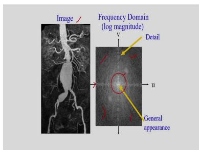
Here, I am showing one example. I have shown one image, that is the image is this, input image. And corresponding to this image I have the Fourier Transform, this is my Fourier Transform. And if I consider this circle, I have shown a circle, the red circle. And if I consider this portion only that means I am only considering the low frequency information, that gives general appearance of the image.
