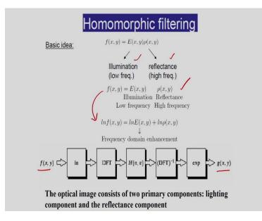
After this I am discussing another filter that is Homomorphic filtering. This filtering technique can be used to improve the appearance of an image by simultaneous intensity range compression and contrast enhancement. Then in this case the main concept is the optical image consists of 2 primary components, what are the primary components? One is the lightening component and another is the reflectance component.
