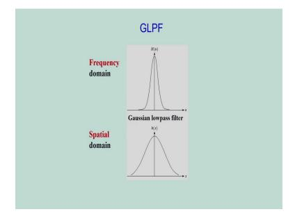
And in this case I have shown the Gaussian low pass filter in frequency domain and after this I have shown the corresponding to spatial domain representation of the Gaussian low pass filter.
