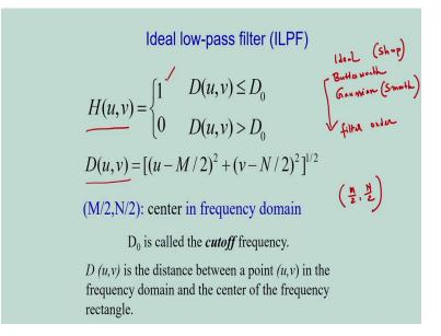
Now, first I am considering the ideal low pass filter. So, before going to the ideal low pass filter in my discussion I will be considering the ideal low pass filter. So, I will be considering the ideal filter, I will be considering the Butterworth filter, also I will be considering the Gaussian filter. In case of the ideal filter that is mainly the sharp filtering, you can consider as a sharp filtering.
