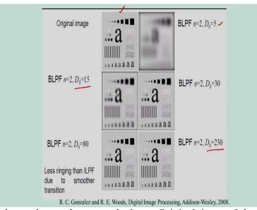
So, in this case I have shown the example here. Original image I have shown, and I am considering the Butterworth low pass filter. The order I am considering n is equal to 2, and I am changing the cutoff frequency, the cutoff frequency is D naught I am changing. The first one is 5, next one is 15, 30, 80, 230 like this. And in this case if you see, if a cutoff frequency is less the blurring will be more. Because of the central lobe of the sinc function.
