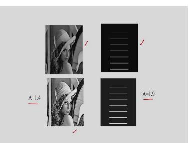
And in this case I can show these two examples. Corresponding to this image I may applying the high boost filter. And in this case I am considering A is equal to 1.4, and corresponding to this I am getting the output image, this. That means I am getting the background information as well as I am sharpening the edges.
