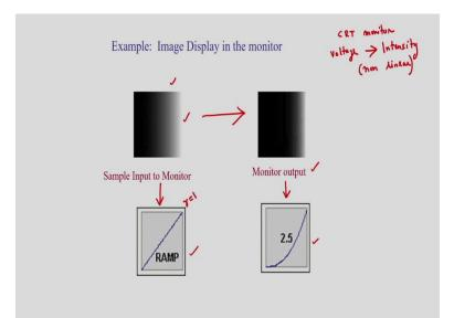
Now, one application of gamma transformation, I can give one example. Suppose in the CRT monitor, the cathode ray tube monitor, what is happening? It is nothing but the voltage is converted into light intensity. That means, I am getting the output in the monitor. Then in this case, it is basically the non-linear. This operation is the non-linear operation. This is non-linear operation. That is the non-linear power function.
