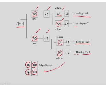
So this concept, I am showing here. So f n is the input image. The two dimensional signal, that is the image I am considering. And I am considering the low pass filter and the high pass filter to get the average value and the detail value. And after this, I am doing the down sampling by 2.
