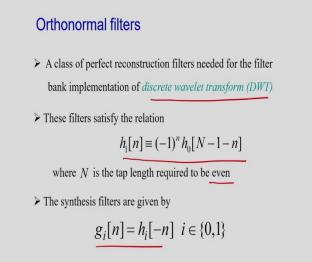
And we are considering a class of perfect reconstruction filters needed for the filter bank implementation. So I have to consider filter banks because I have to decompose the signal for discrete wavelet transformation. For discrete wavelet transformation, we need the filter banks, the low pass filter and the high pass filters.
