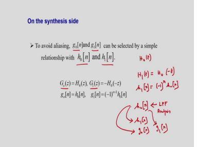
And similarly, for the synthesis side also we need the low pass filter and the high pass filter. So here you can see g naught n, g1 n. g naught n is the low pass filter, that is the synthesis filter. And g1 n is the high pass filter. So from this, you can see, from h naught n, that is, in the time domain, that is, the low pass filter, and h1 n is the high pass filter in the time domain.
