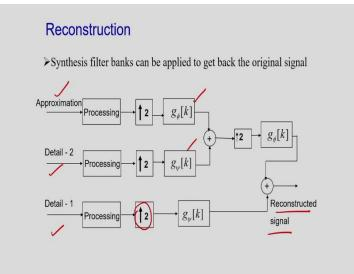
And for the synthesis, for the reconstruction, the opposite is this. Because I have the approximate information, I have the detail information, detail information 1, detail information 2. And you can see, by considering again the filter banks, the low pass filter and the high pass filer, you can reconstruct the signal.
