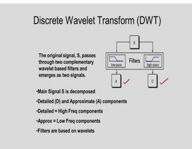
In this figure also I am considering the decomposition of a particular signal, that is the discrete wavelet transformation I am considering. For decomposition of the signal, I am considering the low pass filter and the high pass filter. So I will be getting the approximate component and the detail component. So this is the decomposition of a particular signal.
