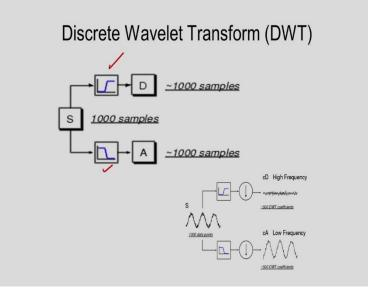
In this case also I am showing one signal, the 1D signal. And I am considering one low pass filter and one high pass filter to get the approximate and the detail components. So, any 1D signal can be decomposed like this. Now, I am discussing the 1D signal that can be extended for 2D signals. Like, in the image we can do the decomposition.
