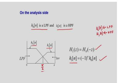
What is a Quadrature Mirror Filter? Here, you can see I am showing the frequency response of the low pass filter and the high pass filter. So, h naught n is the low pass filter and h1 n is the high pass filter. So, how to get the high pass filter? That is nothing but h1 n is the mirror of h naught n. That is, the high pass filter is the mirror of the low pass filter.
