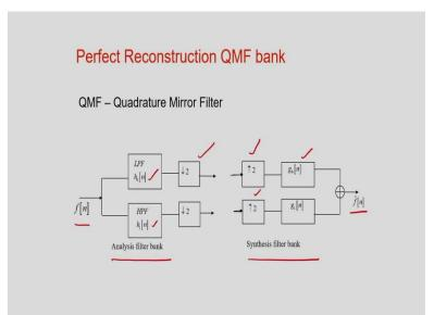
So, this implementation can be done by using two filters, one is the low pass filter, another one is the high pass filter. That means, the decomposition can be done by considering two filters, one is the low pass filter. The low pass filter is h naught n, and high pass filter is h1 n, I am considering.
