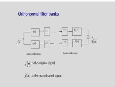
So here, you can see, I am showing the analysis of the signal and also the reconstruction of the signal. So here you can see I am considering the low pass filter h naught n, and high pass filter is h1 n. And I am considering the Quadrature Mirror Filter. So from h naught n you can determine h1 n. So the signal is decomposed by considering this low pass filter and the high pass filter.
