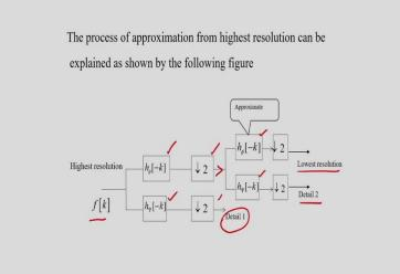
So this multiple level of decomposition we can do by using these filter banks. In this figure, you can see the multiple levels of decompositions I can do. So first, I am considering the signal, the signal is f k, that is of highest resolution. After this, I am considering the low pass filter and the high pass filter. I am determining the approximate value and the detail vale.
