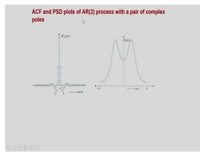
We can plot the ACF and PSD of AR2 process these are the plausibly simulated AR2 process and we see that this is a particular case for complex poles so the autocorrelation behaves like this both positive and negative values are there and power spectrum has a peak this is a negative side of the spectrum so there is a peak corresponding to this point. So, that way you suppose if we have a some dominant frequency component in a random process then we can get it by AR2 spectrum.
