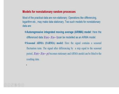
So, far we have discussed how to model WSS random process but most of the practical that there are non stationary operations like differencing logarithm etcetera may be are found to make data stationary. There are different ways to make data stationary to such models for non stationary data. First one is ARIMA model autoregressive integrated moving average model. Here the difference data Xn - Xn - 1 can be modeled as a ARMA model after differencing this data will be fitted into an ARMA model.
