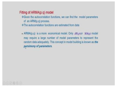
How to fit an ARMA p, q model, so given the autocorrelation functions we can find the model parameters of n ARMA p q process so because of the relationship between the autocorrelation functions and the model parameters we can find out the model parameters. The autocorrelation functions are estimated from data generally autocorrelation functions will be estimated from the data and those autocorrelation functions are used to estimate the model parameters.
