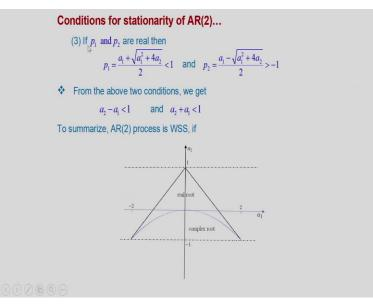
Now condition 3 if p 1 and p 2 are real then both roots p 1 and p 2 both her magnitude of both will be less than 1 now this is the larger root out of 2 this is the larger root therefore its value must be less than 1 and this is the smaller root because this minus sign, so this must be greater than -1 these are both real and from the stability conditions we get this. And from the above two conditions we will get that a 2 - a 1.
