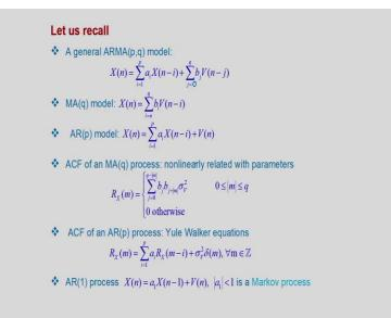
Hello students in this lecture i will discuss linear models of random signals 2. Let us recall a general ARMA p q model is given by Xn is equal to summation ai X of n - i i going from 1 to p plus summation bj a of n - j j going from 0 to q this is an ARMA p q model and we also discuss MA q model that is Xn is equal to summation bi V of n - i i going from 0 to q AR p model autoregressive of order p that is Xn is equal to summation ai X of n - i i going from 1 to p + Vn.
