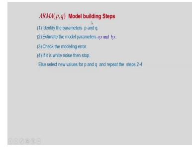
We will broadly describe ARMA p q model building steps, first step is identify the model order parameters p and q. After p and q are identified estimate the model parameters ai's and bi's check for the modeling error, if suppose we will find out the difference between actual sample value and the value predicted by the model. If it is white noise then stop so model building is over else select a new values of p and q and repeat these steps 2 to 4.
