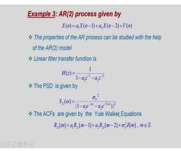
We will consider another example that is AR2 process given by Xn is equal to a1 X of n - 1 + a 2 X over n - 2 plus Vn this is a very good example the properties of AR processes can be studied with the help of this model. Let us see firstly linear filter transfer function corresponding to this process this linear filter transfer function is given by 1 by 1 - a 1 z to the power - 1 - a 2 into z to the power of -2. So, this is an all pole model it has two poles.
