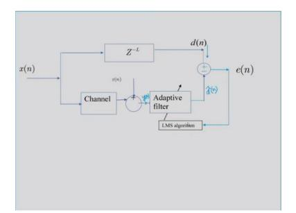
The filter set up is like this the test sequence xn is passed through a delay to the receiver so that where dn is the test sequence, but it is delayed by some amount. Now the test sequence is passed traditional good transfer function we know and then there is a addition of noise so this vn noise is added here and the output is passed to the adaptive filter. The adaptive filter will estimate d hat. So d hat n will be estimated, and the error will pass over to the LMS algorithm.
