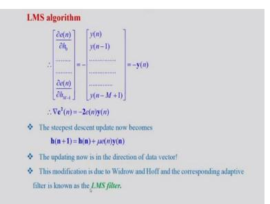
The partial derivative factor is now given by negative of this vector yn yn - 1 up to yn - m + 1 that = - yn vector. Therefore gradient of e square n will be - 2 times en into yn vector from this relationship variant of e square n = 2 times en into this partial derivative vector. So from that we will get that gradient of e square n = -2 times en into yn. This steepest descent update now becomes h of n + 1 = hn + mu times n into yn.
