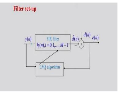
Now we describe the LMS algorithm based adaptive filter set up here yn is the input this is passed through the FIR Wiener filter of step length m - 1 then we will get the estimate of the desired signal and this is the desired signal which we have to decide. So this is positive this one
