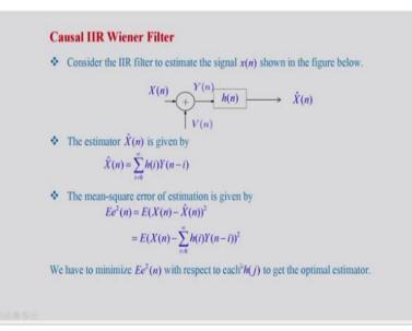
Let us consider this filtering problem; consider the IIR filter to estimate signal xn as shown in figure below, this is the figure here, Xn + Vn that is our observed signal Yn and we apply the IIR Wiener filter with filter coefficient hn to get the estimated signal X hat n, so this is the IIR Wiener filter structure, there are infinite number of coefficients from h0 to h infinity. The
