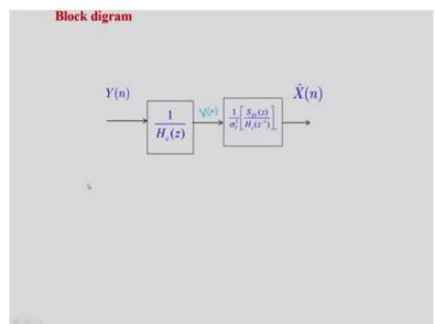
We can represent the procedure in a block diagram; Yn is passed through this filter of transform function 1 by He z to get the innovation process Vn, which is now passed through this filter 1 by sigma v square into the positive part of Sxyz divided by Hz inverse and we will get the estimator X hat n. This is the principle of causal IIR Wiener filter.
