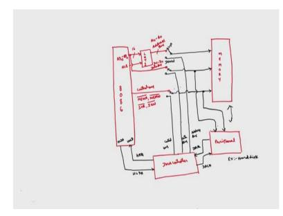
There is a microprocessor so, this can be any microprocessor here I will consider 8086 then we have memory, the same previous diagram I am going to show in detail. We have memory and then we have peripheral, then we need a DMA controller, direct memory access controller.
