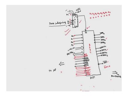
So, if I take the DMA device 8237 or 8237A this is 8237. So, total 40 pins are available ok. So, one is chip select signal for any chip, we will we require a chip select signal then we have the other side. This side is actually we will connect to the peripherals this side, we will connect to microprocessor.
