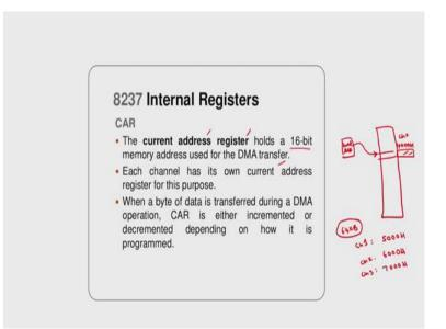
So, first one is a current address register. As I have told so, if we want to transfer the data from peripheral to such as hard disk to memory. So, where does the first byte has to be transferred? What is the address of this one? So, this will be decided by this current address register. This holds 16 bit memory address used for the DMA transfer, the starting address.
