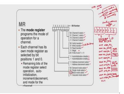
So, I will write the program using this command register after some time, then the mode register. There are two important registers; one is command register, another is mode register. So, mode register as the name implies it will select the mode of operation. So, this will decide the channel to be selected. So, if this is channel 0, 0 0, channel 1, 0 1, channel 2, 1 0, channel 3, 1 1.
