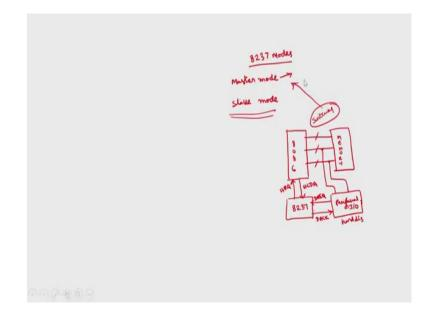
We can operate this in master mode as well as slave mode 8237 modes. In master mode, I have discussed these 7 or 8 steps in the earlier lecture. So, the step by step procedure that follows to operate this 8237 in master mode. In slave mode simply so, this DMA controller will be acts as a slave mode. So, in that case simply this 8086 will be connected to memory address bus data bus control bus.
