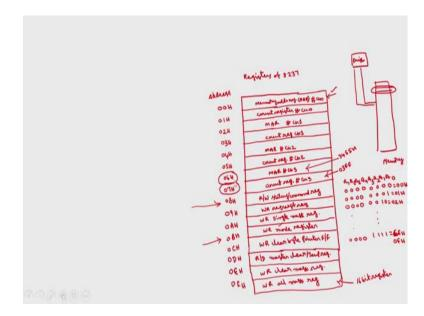
So, the register so, of 8237. Corresponding to each channel we have two registers; one is called memory address register, another is called count register. So, this is memory address register corresponding to channel 0 memory address register, I will call as MAR corresponding to channel 0 and corresponding to this same channel 0 we have count register.
