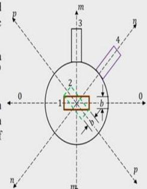
So, in this 4 port circulator, all ports are kept matched, and transmission of power takes place in cyclic order. That means 1 to 2, 2 to 3, 3 to 4, like that. Based on the principle of Faraday rotation, a magnetized ferrite rod is used to provide a 45-degree rotation of the electric field. All 4 ports in the circulator are arranged such that E field is coupled to these ports in numerical order after going through a rotation of 45 degrees in clockwise direction.
