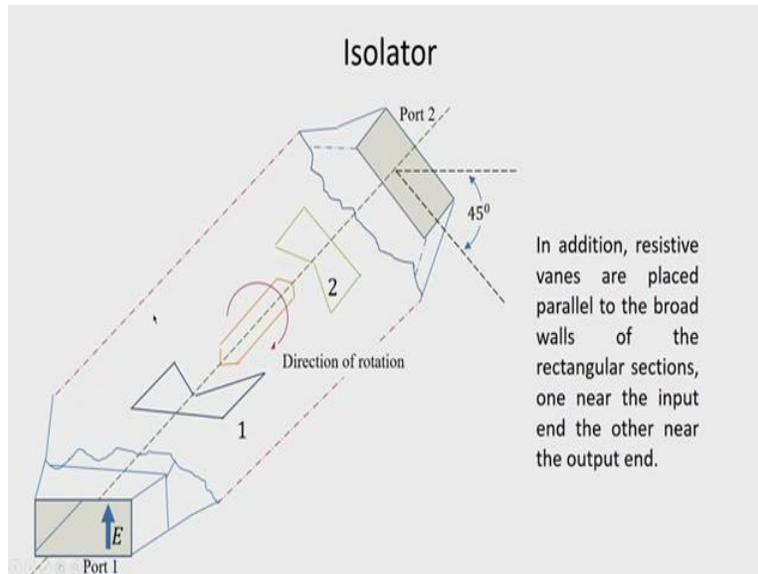
This is illustrated with the diagram shown in the figure. At the input port let us suppose this is the polarization of the wave, now when this propagates and enters the circular section of the waveguide through this transition, this  $TE_{10}$  mode will give rise to  $TE_{11}$  mode in the circular waveguide but its polarization will remain same as before and here this electric field is perpendicular to this resistive vane.
