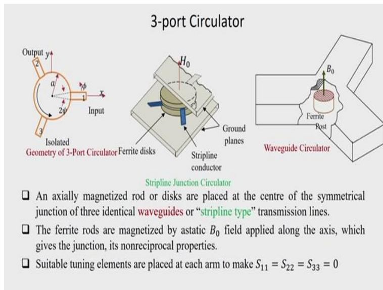
All these S parameter magnitudes will be unity. Now, this type of 3 port circulators can be realized either in the form of stripline junction, in the form of a y junction or in the form of a waveguide circulator. In case of a stripline junction circulator, we have the ground planes on the top and bottom, and between the stripline conductor and the ground plane are the ferrite discs, and the magnetic field is applied along the axis of this disc.
