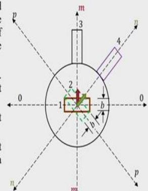
So, referring to this figure, whenever a signal is an incident at port 1, E field vector will in the direction of m, so this is the E field vector. Now, as the wave travels along the magnetic ferrite the
